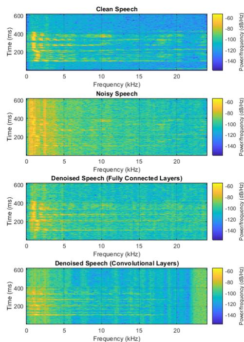
The spectrograms tell us more about how the model is performing at different frequencies. For example, we can see it was particularly effective at removing noise at lower frequencies, where most of the speech spectrum is concentrated.
