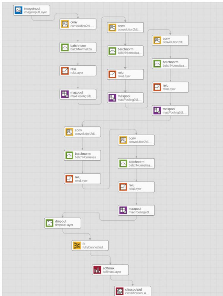
It is up to the designer of the network to determine how many iterations of convolution, batch normalization, and ReLU to perform, but keep in mind that the more complex the network, the more data required to train and test it.
