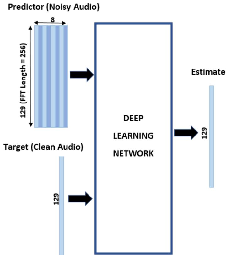
*The predictor input consists of eight consecutive noisy STFT vectors, so each STFT output estimate is computed based on the current noisy STFT and the seven previous noisy STFT vectors for more context.*
