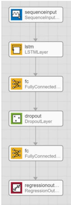
An LSTM is a good fit for this kind of application because it can learn dependencies between time steps of sequence data. Sensors are often interconnected, and an event that happened two cycles ago can affect the future performance of the system.
