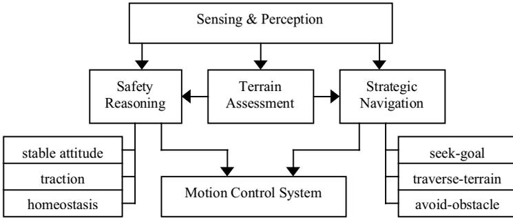
**Figure 11.2:** Modular System Diagram.
