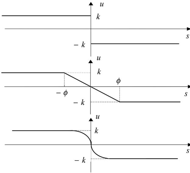
**Figure 12.2:** Various Sliding Mode Controllers.
