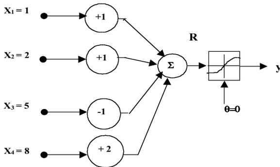
**Figure 2.9:** Neuron Structure of Example 2.1.
