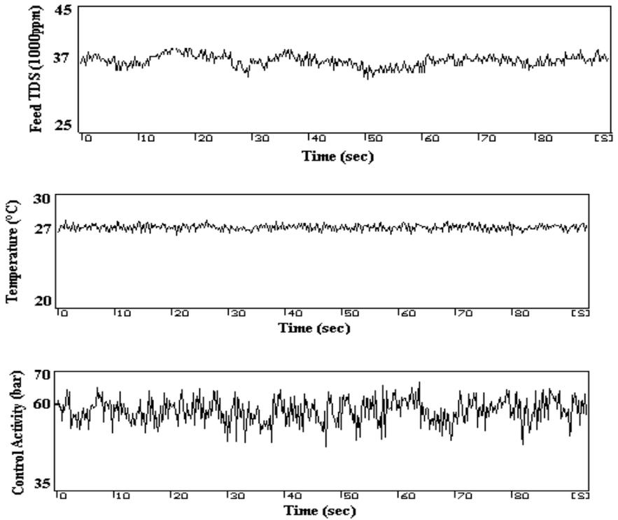
**Figure 15.25:** Feed Conductivity (Top), Temperature (Middle), and Control Activity of High Pressure Pump (Bottom).
