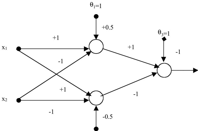
**Figure 2.21:** Neural Network Architecture for Example 2.3.
