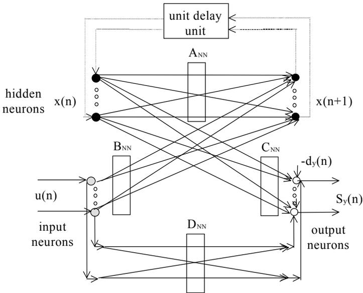
**Figure 5.2:** The Network Structure Designed for System Identification.
