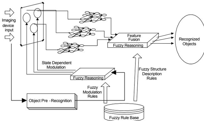
**Figure 16.1:** A Prototype of Object Recognition by Neural Feature Extractions and Fuzzy Structural Description.
