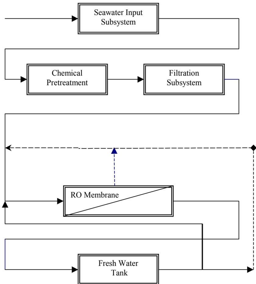
**Figure 15.17:** Process Layout of the Implemented RO System.
