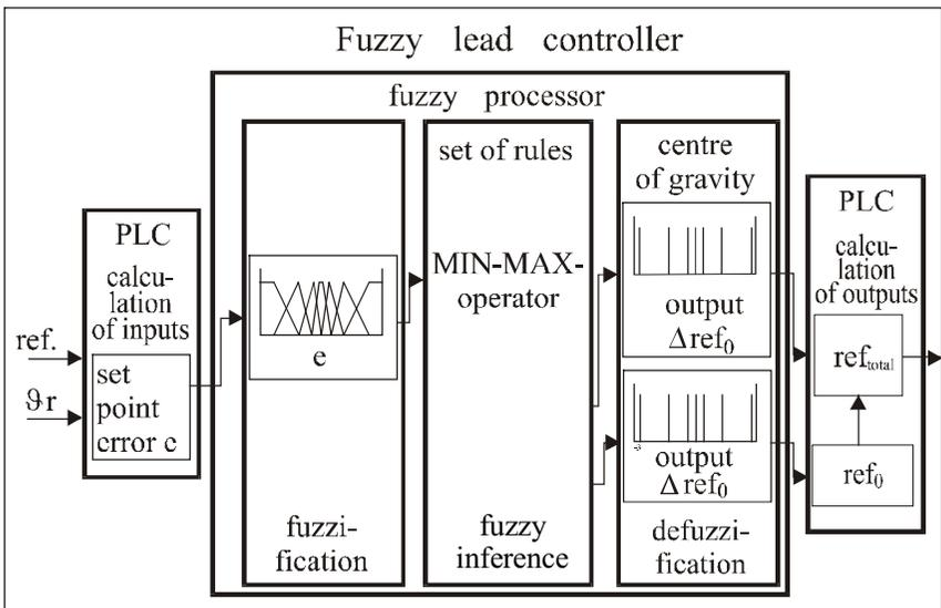
**Figure 13.7:** The Lead Controller with Fuzzy PI Characteristics.
