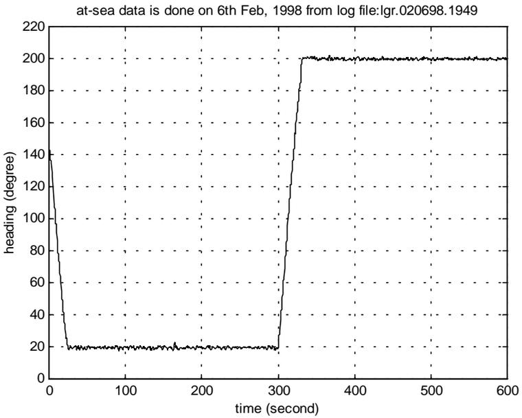
**Figure 12.13:** At Sea Test for Sliding Mode Fuzzy Heading Controller.
