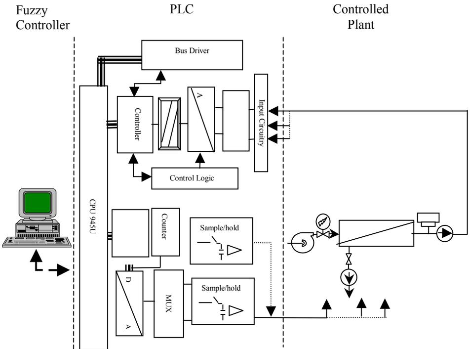
Figure 15.15: Hardware Setup for the RO Plant.
