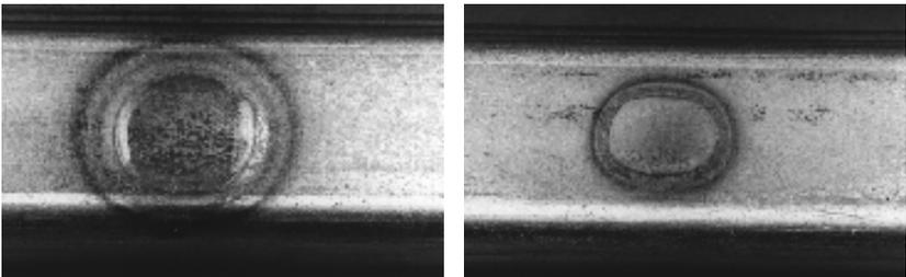
**Figure 18.7:** Example of a Good (Left) and Poor (Right) Welding Spot.
