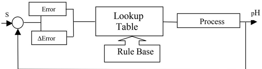
**Figure 15.20:** Block diagram of the Fuzzy Controller for the Chemical.
