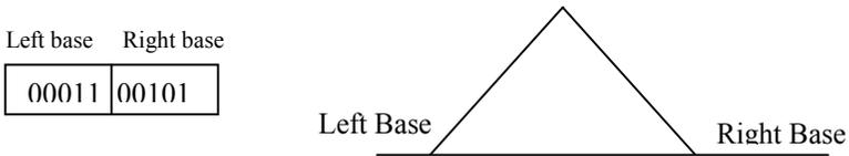
**Figure 19.4:** Symmetric Triangular Membership Function and Its MFC.
