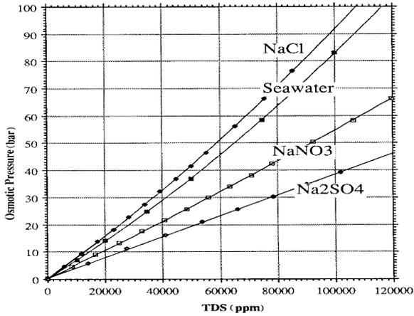
**Figure 15.1:** Osmotic Pressures of Different Solutions at 25°C (Courtesy of The DOW Chemical Company, 1993).
