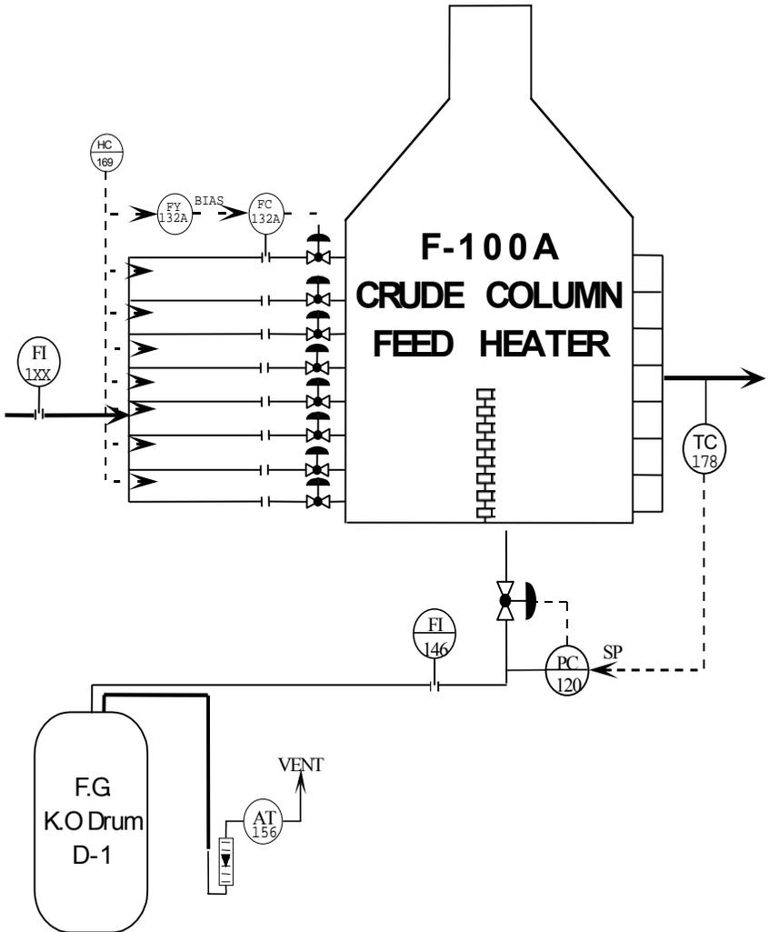
**Figure 7.3:** Block Diagram of Fuel Gas Supply System.
