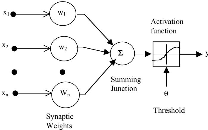
**Figure 2.2:** Basic Elements of an Artificial Neuron.
