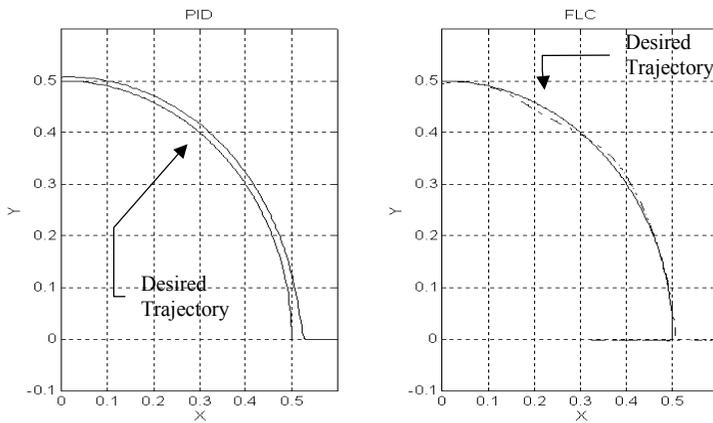
**Figure 14.27:** Case 5: P-D vs. FLC with Calculated Inverse (Trajectory Plot).
