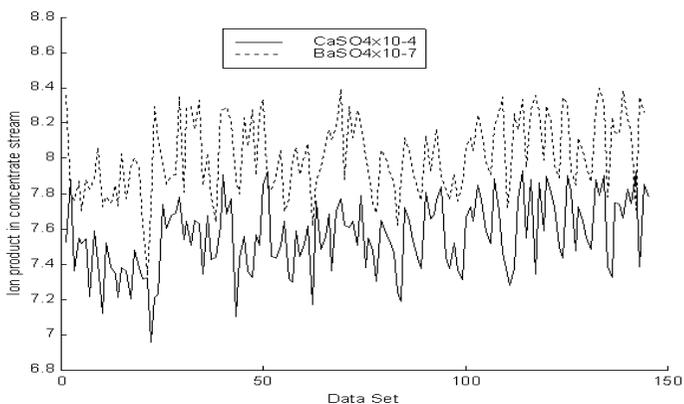
**Figure 15.14:**  $IP_c$  for CaSO<sub>4</sub> and BaSO<sub>4</sub> in Concentrate Stream
