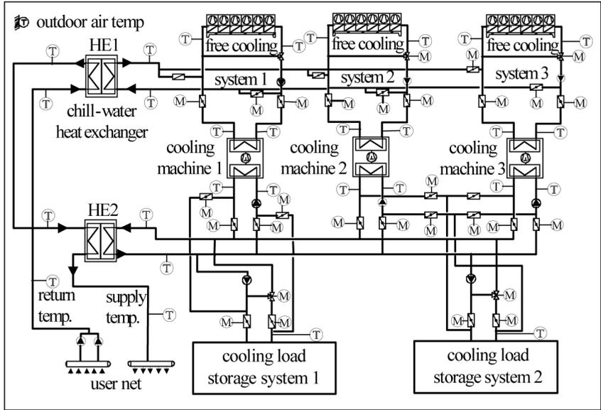
**Figure 13.10:** Schematic Diagram of the Chilling System.
