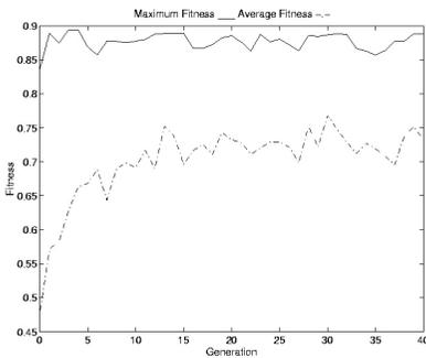
**Figure 19.22:** Plot of Maximum and Average Fitness Values of GA for a DC Motor.
