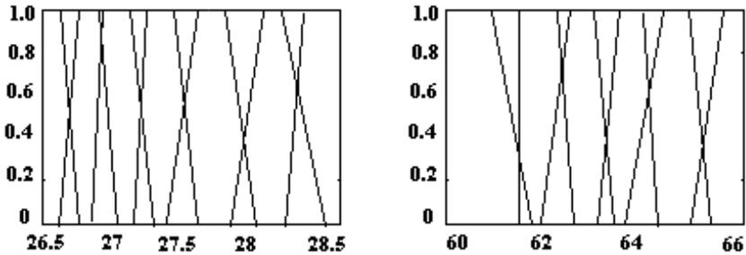
**Figure 15.33:** Final Membership Functions Using ANFIS for Temperature (Left), and Feed Pressure (right).
