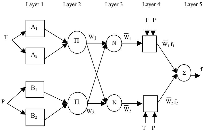
**Figure 14.1:** ANFIS Architecture for a Two-Input System.
