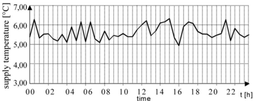
Figure 13.14. Course of Supply Temperature with FLC Operated System.
