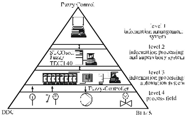
**Figure 13.1:** Building Energy Management System with Fuzzy Control.
