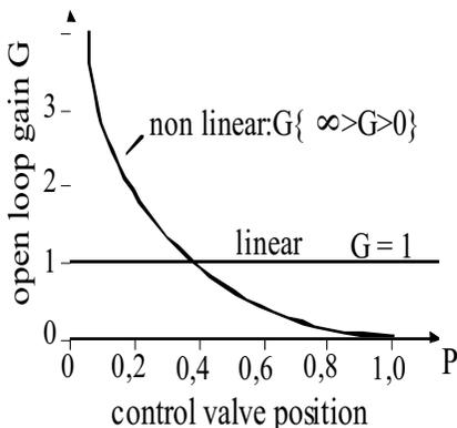
**Figure 13.5:** Nonlinear Open Loop Gain of the Heat Exchanger.
