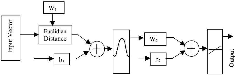
**Figure 15.4:** RBFN Network Architecture.
