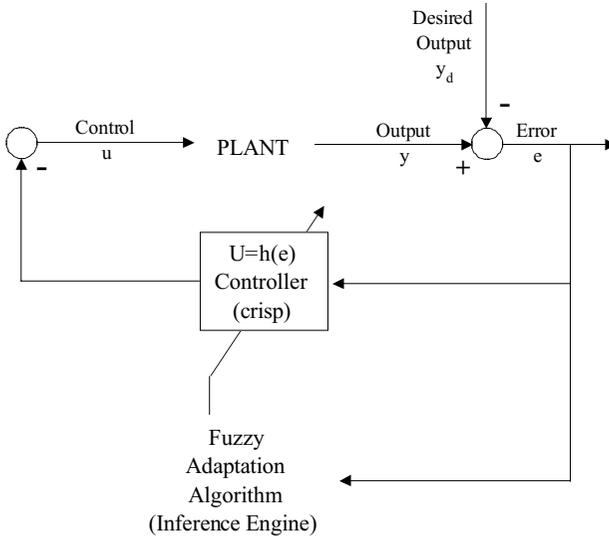
**Figure 10.3:** An Adaptive (Tuner) Fuzzy Control System, Fuzzification.
