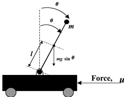
**Figure 10.6:** Inverted Pendulum.
