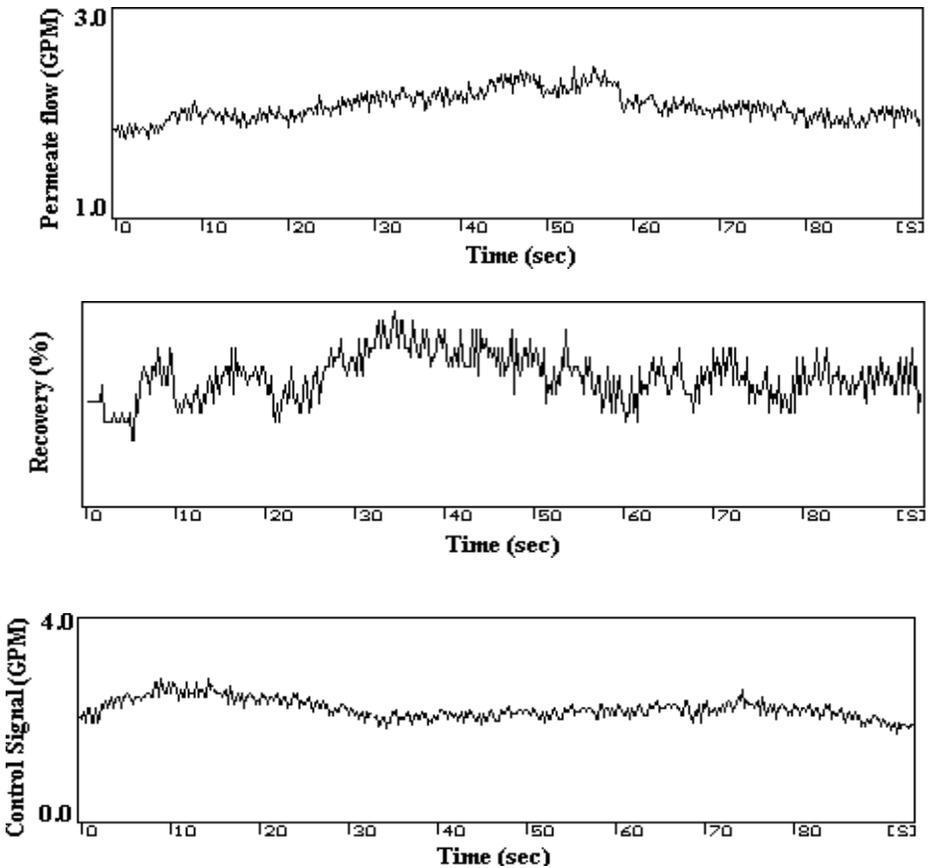
**Figure 15.29:** Effect of High Permeate Flow on Recovery and Motor Speed Control Signal.
