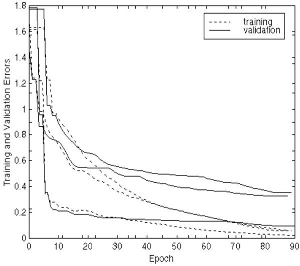
**Figure 15.7:** LMS and Corresponding Validation Curves for Selected Values of Learning Rate (0.05 Top Curves, 0.1 Middle Curves, 0.5 Bottom Curves).
