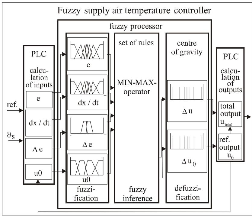
**Figure 13.6:** Fuzzy PID Supply Air Temperature Controller.
