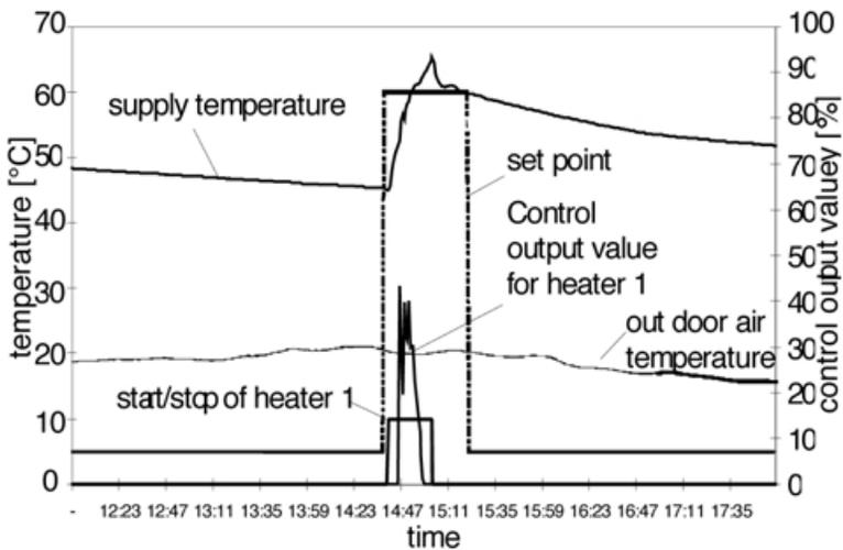
Figure 13.22: Heating System's Behavior Operated by Fuzzy Control.
