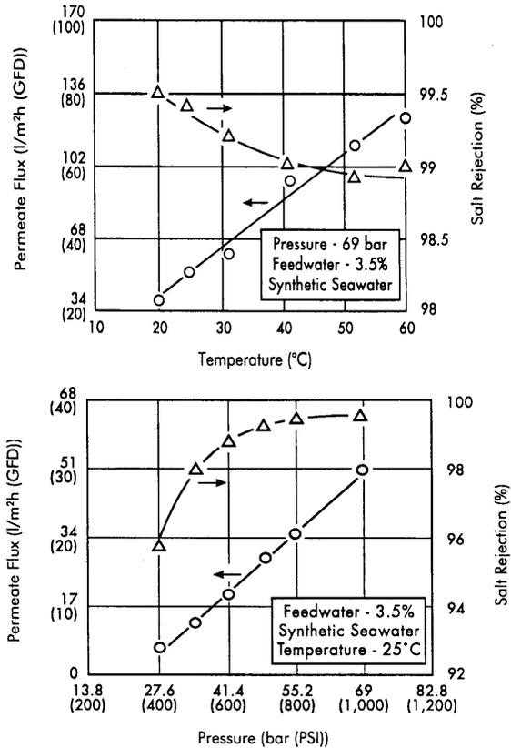
**Figure 15.2:** Effects of Feed Temperature and Pressure on Permeate Flux and Salt Rejection (Courtesy of The Dow Chemical Company, 1993).
