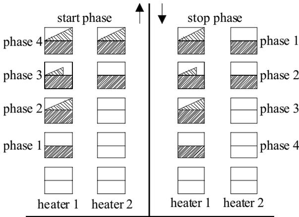
**Figure 13.18:** Operation Strategy for a Cascade Heating Center.
