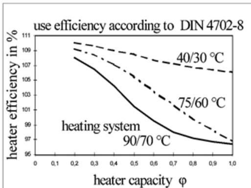
**Figure 13.16:** Thermal Efficiency of the Heating System.
