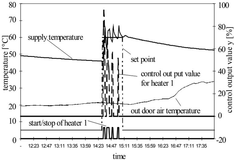
Figure 13.21: Heating System's Behavior Operated by Digital Control.
