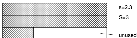
Fig. 1.5. Mapping an array onto a store
