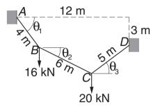
The 15-m cable is suspended from *A* and *D* and carries concentrated loads at *B* and *C*. The vertical equilibrium equations of joints *B* and *C* are
