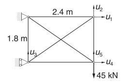
The displacement formulation for a plane truss is similar to that of a mass-spring system. The differences are: (1) the stiffnesses of the members are  $k_i = (EA/L)_i$ ,
