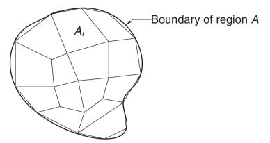
Figure 6.6. Finite element model of an irregular region.
