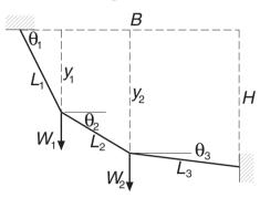
A cable supported at the ends carries the weights  $W_1$  and  $W_2$ . The potential energy of the system is
