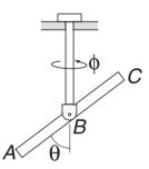
The bar *ABC* is attached to the vertical rod with a horizontal pin. The assembly is free to rotate about the axis of the rod. Neglecting friction, the equations of motion of the system are
