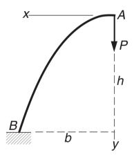
A uniform beam forms the semiparabolic cantilever arch *AB*. The vertical displacement of *A* due to the force *P* can be shown to be
