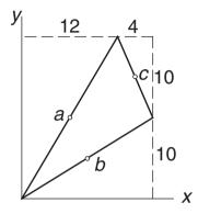
**Solution** Because f(x, y) is quadratic, quadrature over the three integration points shown in Fig. 6.10(b) will be sufficient for an "exact" result. The integration points lie in the middle of each side; their coordinates are (6, 10), (8, 5), and (14, 15). The area of the triangle is obtained from Eq. (6.49):
