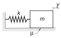
Consider the mass–spring system where dry friction is present between the block and the horizontal surface. The frictional force has a constant magnitude  $\mu mg$ ( $\mu$  is the coefficient of friction) and always opposes the motion. The differential equation for the motion of the block can be expressed as
