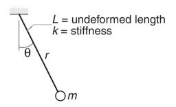
The mass *m* is suspended from an elastic cord with an extensional stiffness *k* and undeformed length *L*. If the mass is released from rest at  $\theta = 60^{\circ}$  with the cord unstretched, find the length *r* of the cord when the position  $\theta = 0$  is reached for the first time. The differential equations describing the motion are
