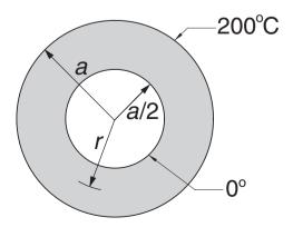
The thick cylinder conveys a fluid with a temperature of  $0^{\circ}$ C. At the same time the cylinder is immersed in a bath that is kept at 200°C. The differential equation and the boundary conditions that govern steady-state heat conduction in the cylinder are
