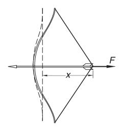
5. The following table gives the pull *F* of the bow as a function of the draw *x*. If the bow is drawn 0.5 m, determine the speed of the 0.075-kg arrow when it leaves the bow. *Hint*: the kinetic energy of the arrow equals the work done in drawing the bow; that is,  $mv^2/2 = \int_0^{0.5m} F \, dx$ .
