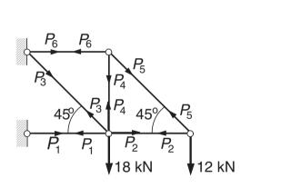
In the *force formulation* of a truss, the unknowns are the member forces  $P_i$ . For the statically determinate truss shown, the equilibrium equations of the joints are
