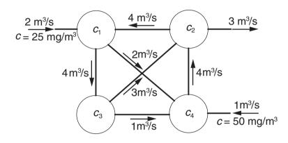
Four mixing tanks are connected by pipes. The fluid in the system is pumped through the pipes at the rates shown in the figure. The fluid entering the system contains a chemical of concentration *c* as indicated. The rate at which the mass of the chemical changes in tank *i* is
