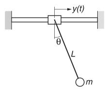
The pendulum is suspended from a sliding collar. The system is at rest when the oscillating motion  $y(t) = Y \sin \omega t$  is imposed on the collar, starting at t = 0. The differential equation describing the motion of the pendulum is
