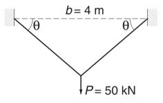
Each member of the truss has a cross-sectional area *A*. Find *A* and the angle  $\theta$  that minimize the volume
