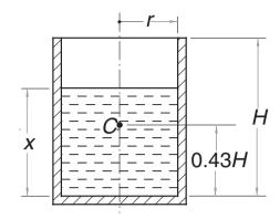
The cylindrical vessel of mass *M* has its center of gravity at *C*. The water in the vessel has a depth *x*. Determine *x* so that the center of gravity of the vessel–water combination is as low as possible. Use M = 115 kg, H = 0.8 m, and r = 0.25 m.
