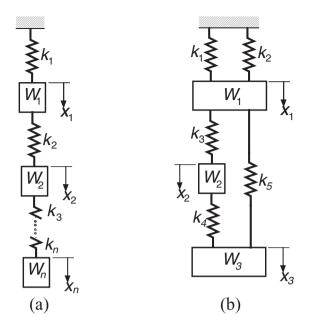
13. ■ The displacement formulation for the mass-spring system shown in Fig. (b) results in the following equilibrium equations of the masses:
