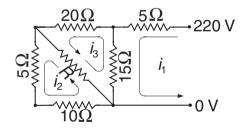
The electrical network shown can be viewed as consisting of three loops. Applying Kirchoff's law ( $\sum$ voltage drops =  $\sum$ voltage sources) to each loop yields the following equations for the loop currents  $i_1$ ,  $i_2$ , and  $i_3$ :
