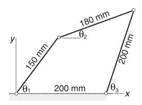
The three angles shown in the figure of the four-bar linkage are related by
