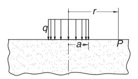
The figure shows an elastic half-space that carries uniform loading of intensity q over a circular area of radius a. The vertical displacement of the surface at point P can be shown to be
