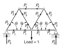
The force formulation of the symmetric truss shown results in the joint equilibrium equations
