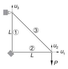
The displacement formulation of the truss shown results in the following simultaneous equations for the joint displacements **u**:
