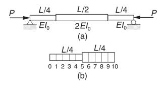
The simply supported column in Fig. (a) consists of three segments with the bending rigidities shown. If only the first buckling mode is of interest, it is sufficient to model half of the beam as shown in Fig. (b). The differential equation for the lateral displacement u(x) is
