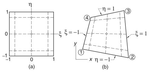
Figure 6.7. Mapping a quadrilateral into the standard rectangle.
