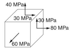
The stress matrix (tensor) corresponding to the state of stress shown is
