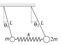
The two pendulums are connected by a spring that is undeformed when the pendulums are vertical. The equations of motion of the system can be shown to be
