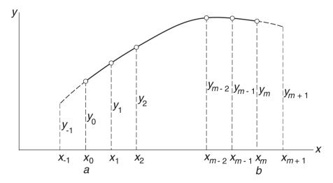
Figure 8.1. Finite difference mesh.
