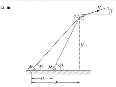
The radar stations *A* and *B*, separated by the distance a = 500 m, track the plane *C* by recording the angles  $\alpha$  and  $\beta$  at 1-second intervals. If three successive readings are
