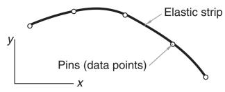
Figure 3.6. Mechanical model of natural cubic spline.
