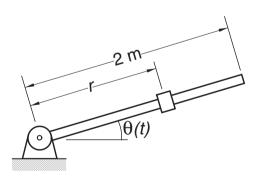
The system consisting of a sliding mass and a guide rod is at rest with the mass at r = 0.75 m. At time t = 0, a motor is turned on that imposes the motion  $\theta(t) = (\pi/12) \cos \pi t$  on the rod. The differential equation describing the resulting motion of the slider is
