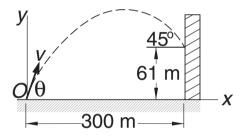
A projectile is launched at *O* with the velocity v at the angle  $\theta$  to the horizontal. The parametric equation of the trajectory is
