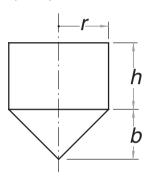
The cylindrical container has a conical bottom and an open top. If the volume V of the container is to be 1.0 m<sup>3</sup>, find the dimensions r, h, and b that minimize the surface area S. Note that
