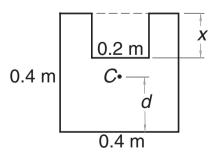
Determine *x* that minimizes the distance *d* between the base of the area shown and its centroid *C*.
