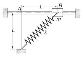
The sliding weight of mass *m* is attached to a spring of stiffness *k* that has an undeformed length *L*. When the mass is released from rest at *B*, the time it takes to reach *A* can be shown to be  $t = C\sqrt{m/k}$ , where
