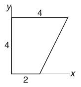
6. Compute  $\int \int_A x \, dx \, dy$  over the quadrilateral region shown by first mapping it into the "standard" rectangle and then integrating analytically.
