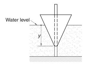
The conical float is free to slide on a vertical rod. When the float is disturbed from its equilibrium position, it undergoes oscillating motion described by the
