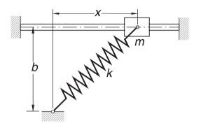
The mass *m* is attached to a spring of free length *b* and stiffness *k*. The coefficient of friction between the mass and the horizontal rod is  $\mu$ . The acceleration of the mass can be shown to be (you may wish to prove this)  $\ddot{x} = -f(x)$ , where
