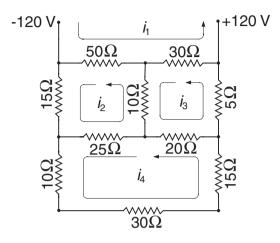
Determine the loop currents  $i_1$  to  $i_4$  in the electrical network shown. 19. Consider the *n* simultaneous equations  $A\mathbf{x} = \mathbf{b}$ , where
