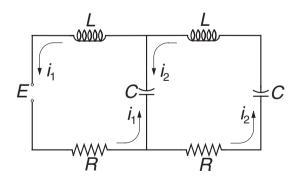
The constant voltage source of the circuit shown is turned on at t = 0, causing transient currents  $i_1$  and  $i_2$  in the two loops that last about 0.05 s. Plot these currents from t = 0 to 0.05 s, using the following data: E = 9 V,  $R = 0.25 \Omega$ ,
