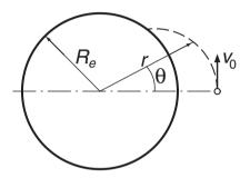
A spacecraft is launched at the altitude H = 772 km above the sea level with the speed  $v_0 = 6700$  m/s in the direction shown. The differential equations describing the motion of the spacecraft are
