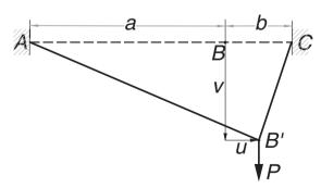
The elastic cord ABC has an extensional stiffness k. When the vertical force P is applied at B, the cord deforms to the shape AB'C. The potential energy of the
