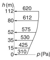
The pressure of wind was measured at various heights on a vertical wall, as shown on the diagram. Find the height of the pressure center, which is defined as
