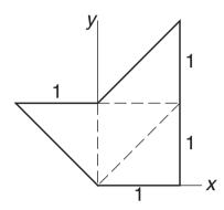
Write a program to evaluate  $\int \int_A f(x, y) dx dy$  over an irregular region that has been divided into several triangular elements. Use the program to compute  $\int \int_A xy(y - x) dx dy$  over the region shown.
