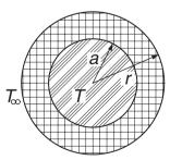
A wire carrying an electric current is surrounded by rubber insulation of outer radius r. The resistance of the wire generates heat, which is conducted through the insulation and convected into the surrounding air. The temperature of the
