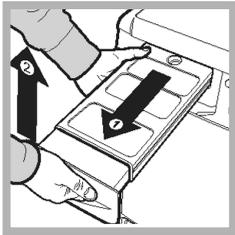
Pull the container out of the dryer and remove either the small or large cap and empty it into a sink or other suitable drain. Refit the cap and replace the container securely.
