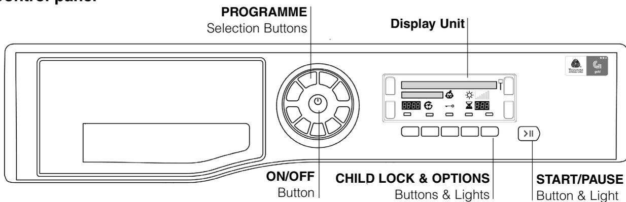
The **ON/OFF** button - if pressed when the dryer is running: If the display shows **TURNING OFF** the dryer stops. If the display shows **PRESS AND HOLD** hold the button and the display counts down 3, 2, 1 and then stops. Press and hold again for more than 3 seconds, the display briefly shows **POWER ON**.
