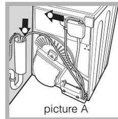
Remove the existing hose from position shown in picture A.
