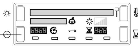
The display counts down the minutes of the delay period after the Start/Pause button
