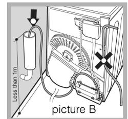
Then fit a suitable length of hose to position shown in picture B.
