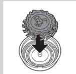
**5** After cleaning, place the cutter back into the guard.
