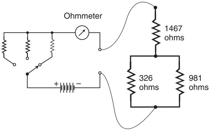
**Figure DC11-6** Resistive network with 1467 ohms in series with a parallel combination of 326 ohms and 981 ohms.
