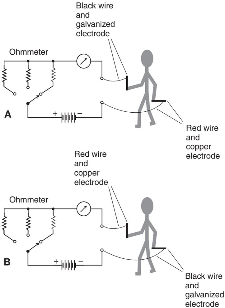
**Figure DC6-2** Try to measure your body resistance with the arrangement you used to measure current in Experiment DC5, as shown at A. Then try the same test with the meter probe wires reversed, as shown at B.
