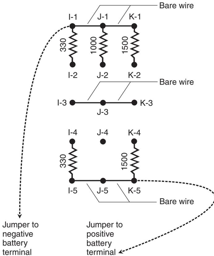
**Figure DC12-1** Arrangement of resistors on breadboard for demonstration of Kirchhoff's current law. All resistance values are in ohms. Solid dots indicate breadboard terminals. Solid lines show interconnections with bare copper wire. Dashed lines indicate jumpers.
