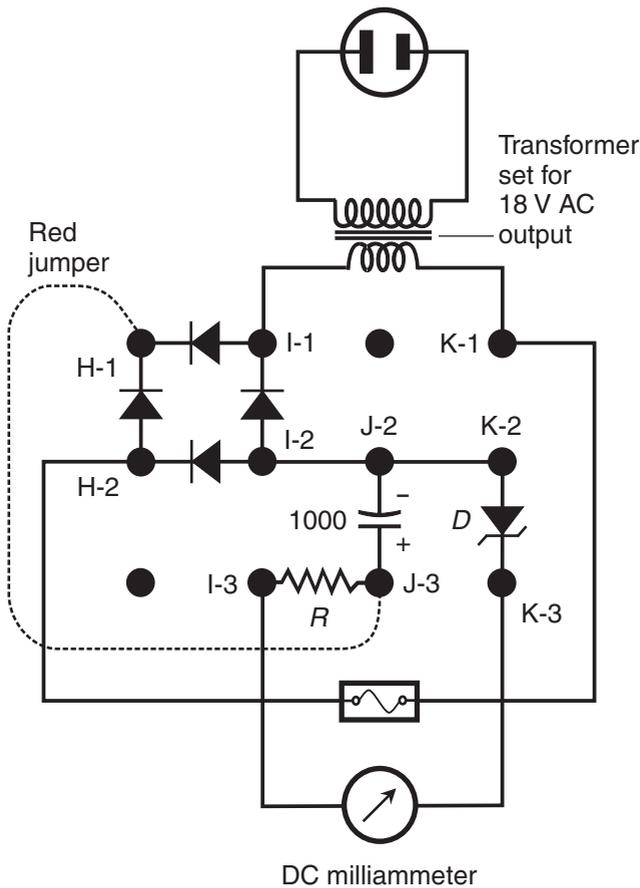
Figure AC16-2 Measurement of the current through the diode and the limiting resistor under no-load conditions.
