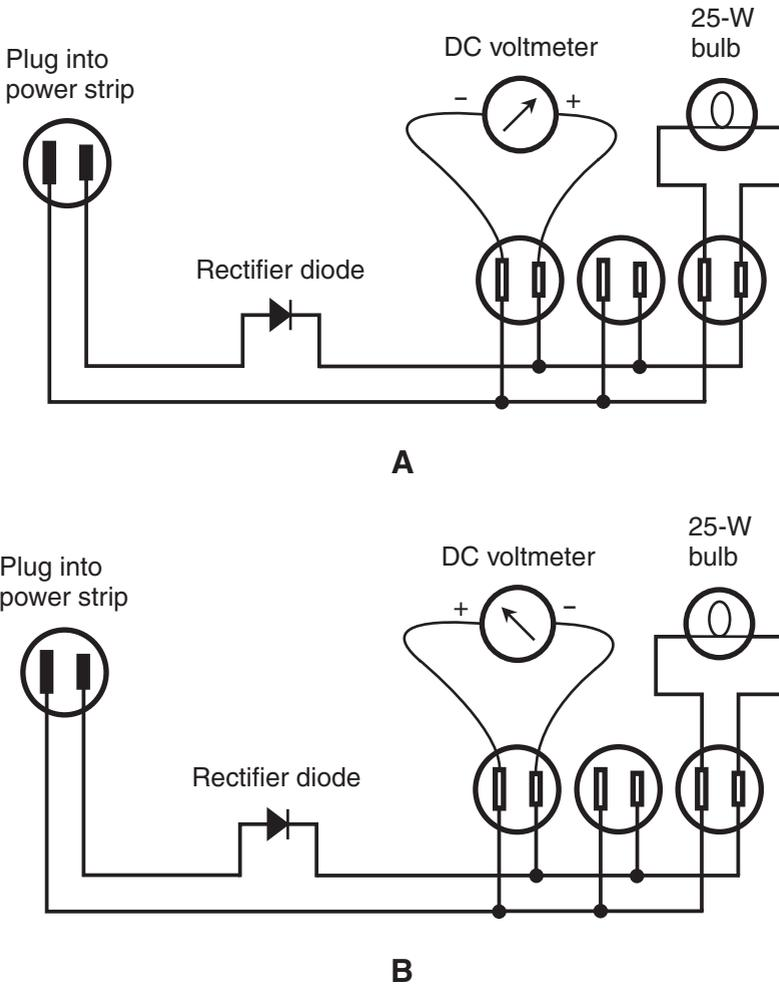
**Figure AC4-3** At A, measurement of the effective DC voltage with the meter polarity matching the rectifier output polarity. The meter shows a positive value. At B, measurement of the effective DC voltage with the meter polarity reversed. The meter displays a negative value, but the absolute voltage is the same as before.
