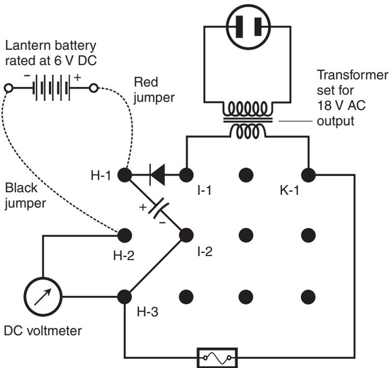
**Figure AC10-3** Measurement of the open-circuit filtered DC output voltage from the transformer-diode-capacitor-battery combination with the battery connected “backward” so its voltage subtracts from the power-supply voltage.
