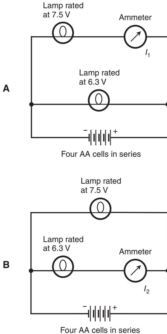
**Figure DC21-1** At A, measurement of current  $I_1$  through the “farther-from-battery” of two dissimilar lamps in parallel (called F, rated at 7.5 V). At B, measurement of current  $I_2$  through the “closer-to-battery” lamp (called C, rated at 6.3 V).
