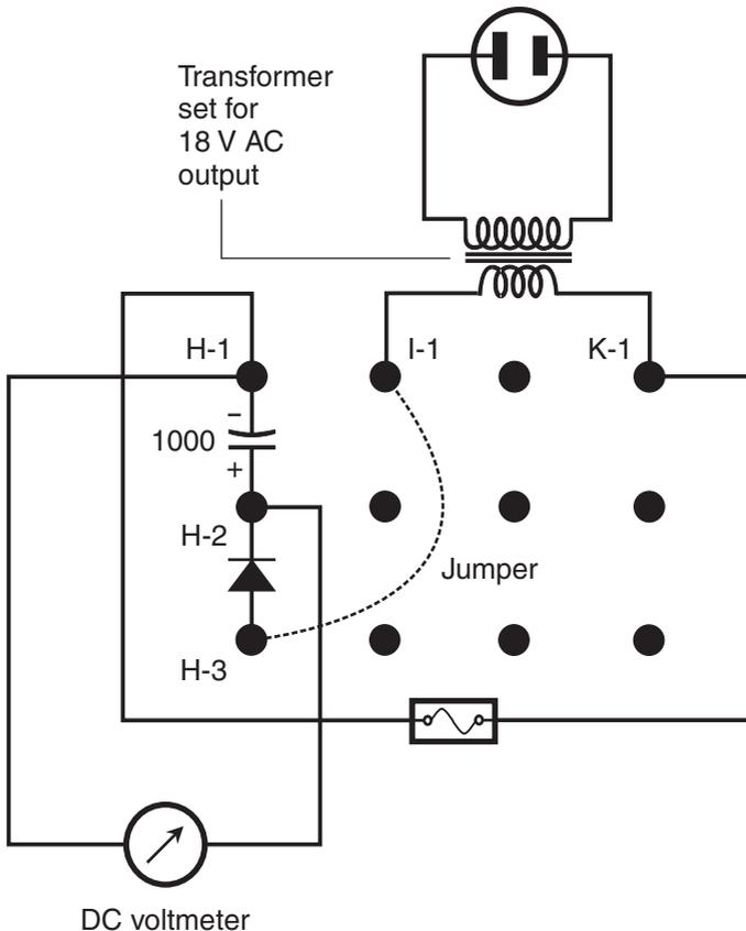
**Figure AC8-1** *Addition of a filter capacitor to the half-wave rectifier circuit, and measurement of the open-circuit filtered DC voltage across the capacitor. The value (1000) is stated in microfarads ( $\mu\text{F}$ ). Pay careful attention to the diode and capacitor polarities! The jumper can serve as a “switch” for the output circuit.*
