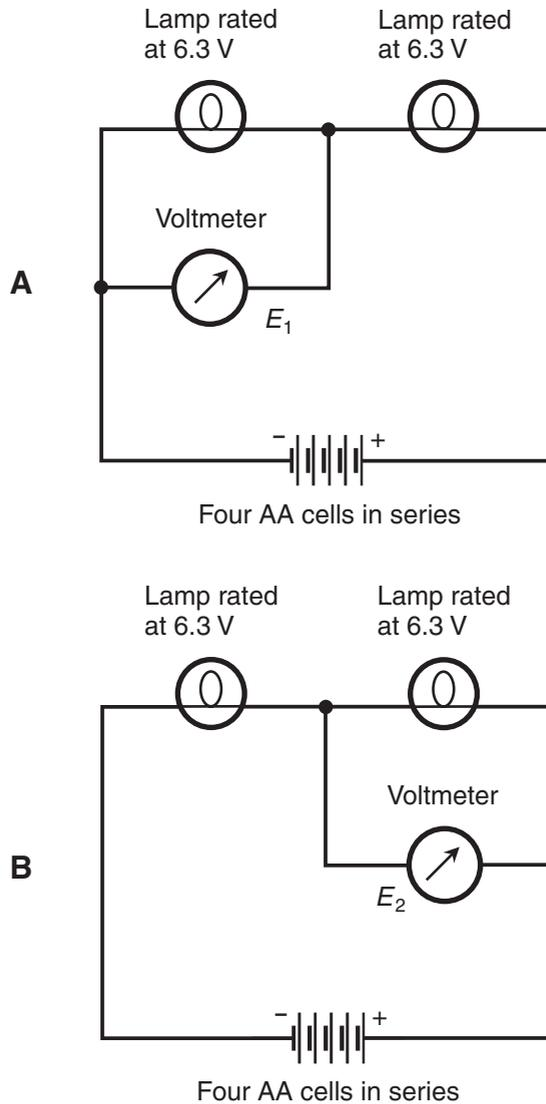
**Figure DC18-1** At A, measurement of voltage  $E_1$  across the more negative of two "identical" lamps in series (called  $N$ , rated at 6.3 V). At B, measurement of voltage  $E_2$  across the more positive lamp (called  $P$ , also rated at 6.3 V).
