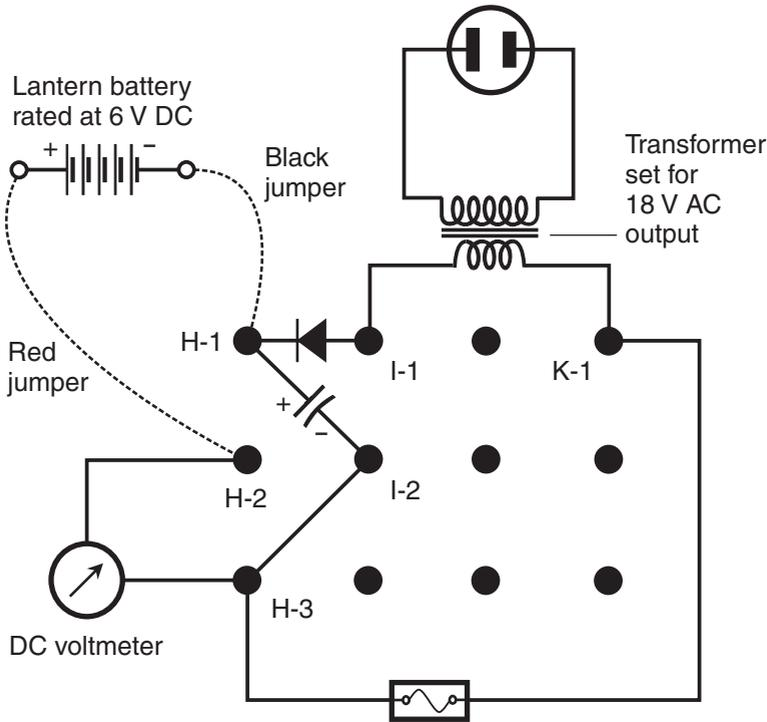
**Figure AC10-2** *Measurement of the open-circuit filtered DC output voltage from the transformer-diode-capacitor-battery combination with the battery connected “forward” so its voltage adds to the power-supply voltage.*
