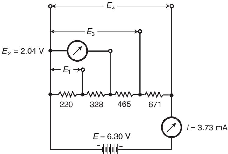
**Figure DC14-3** Network for testing the operation of a resistive voltage divider. All resistance values are in ohms. The battery voltage  $E$ , the voltage across the first and second resistors, and the resistances are those I measured.
