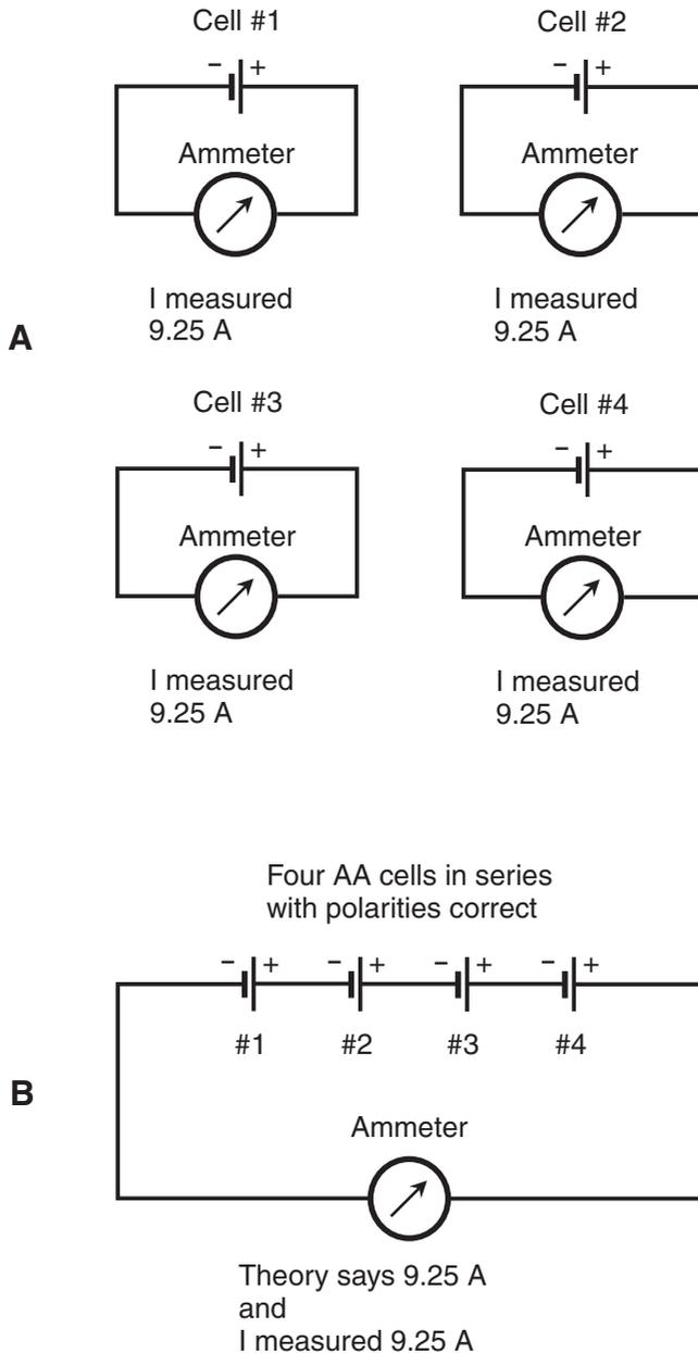
**Figure DC3-1** *I short-circuited four different AA cells with an ammeter, and estimated that each cell produced 9.25 A as shown at A. Then I connected the cells in series so that they all worked together, shorted the combination with the ammeter, and got 9.25 A again as shown at B.*
