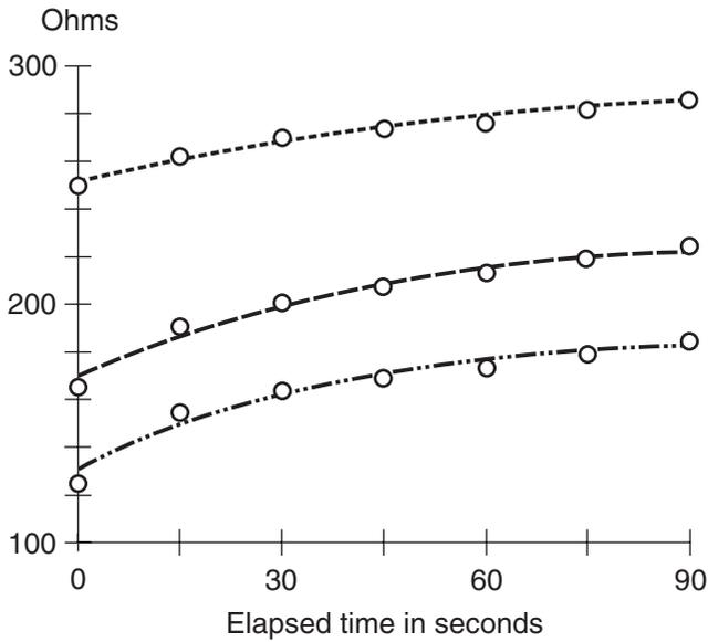
**Figure DC7-2** At A, the arrangement for measuring the resistance of water with salt (sodium chloride) fully dissolved. At B, the resistances I observed over a span of 90 seconds. Upper (short-dashed) curve: 0.5 teaspoon of salt. Middle (long-dashed) curve: 1.0 teaspoon of salt. Lower (dashed-and-dotted) curve: 1.5 teaspoons of salt.
