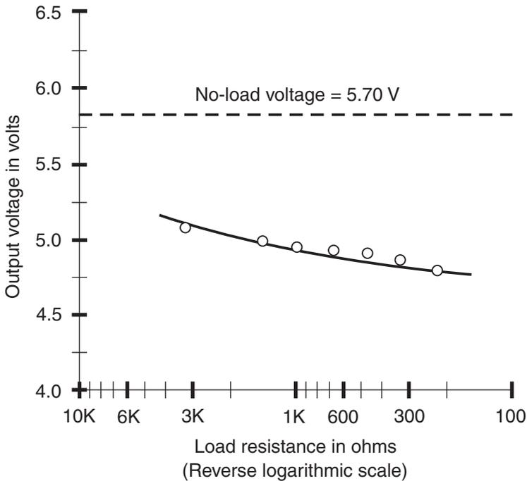
**Figure DC15-4** *Output voltage versus load resistance for the diode-based voltage reducer. These are my results. The dashed line shows the open-circuit (no-load) voltage. Open circles show measured voltages under various loads. The solid curve approximates the circuit's characteristic function.*
