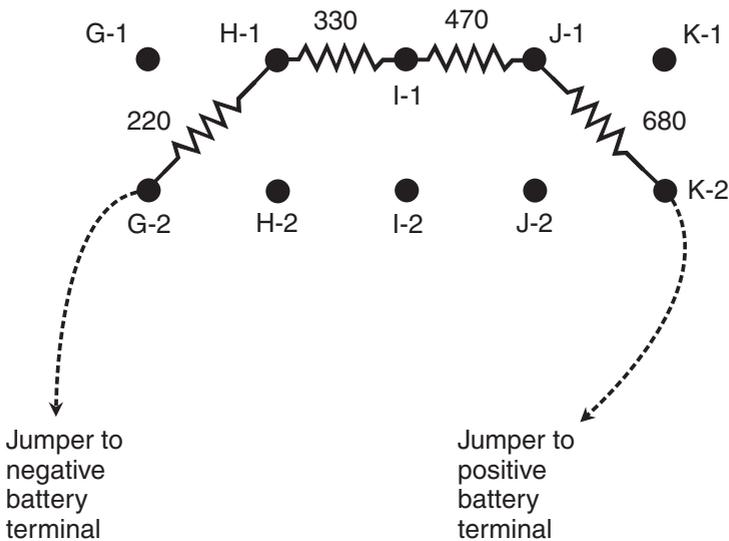
**Figure DC13-2** Suggested arrangement of resistors on breadboard for demonstration of Kirchhoff's voltage law. All resistance values are in ohms. Solid dots indicate terminals. Dashed lines indicate jumpers.
