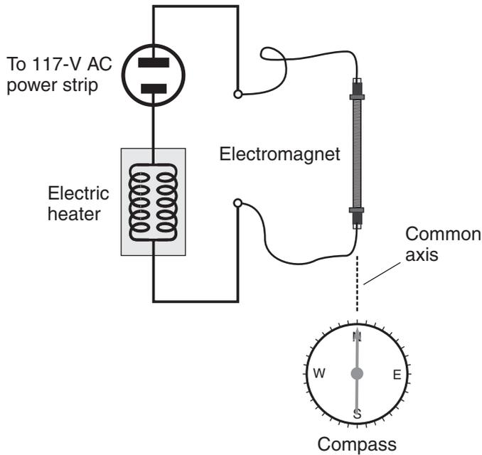
**Figure MAG13-2** *Compass near the end of an electromagnet. The rod and the compass needle should lie along a common axis with the electromagnet powered-down. What will happen when you supply the coil with AC?*
