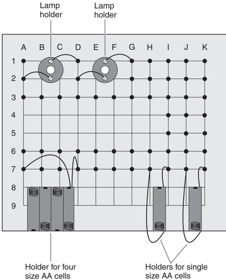
**Figure DC1-1** Layout of the breadboard for DC experiments. I used a “12-in” pine board (actually 10.8 in wide) with a thickness “ $\frac{3}{4}$  in” (actually about 0.6 in), cut to a length of 12.5 in. Solid dots show the positions of the nails. Grid squares measure 1 in by 1 in.
