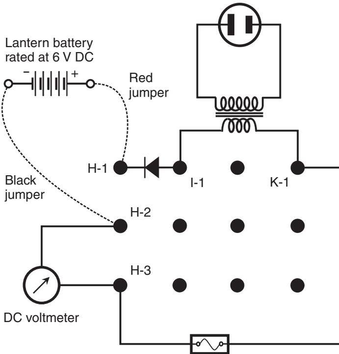
**Figure AC9-3** Measurement of the open-circuit pulsating DC output voltage from the transformer-diode-battery combination with the battery connected “backward” so its voltage subtracts from the rectified voltage.
