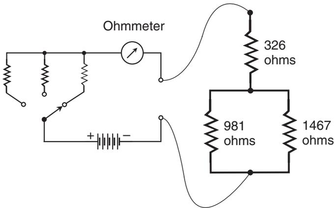
Figure DC11-4 Resistive network with 326 ohms in series with a parallel combination of 981 ohms and 1467 ohms.
