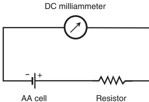
**Figure DC8-1** *To measure the current that a known voltage drives through a known resistance, simply connect the voltage source, the resistor, and the meter in series.*
