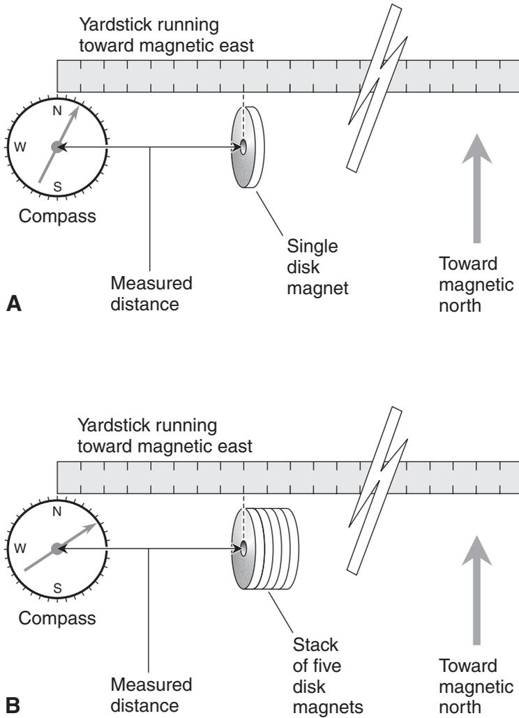
**Figure MAG 3-1** At A, the arrangement for testing the effect of a single disk magnet on a compass. At B, the arrangement for testing the effect of a stack of five disk magnets. Distances should be measured between the center of the compass and center of the nearest magnet face.
