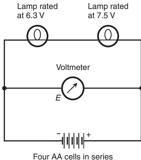
**Figure DC19-2** *Measurement of voltage  $E$  across the combination of two dissimilar lamps in series.*
