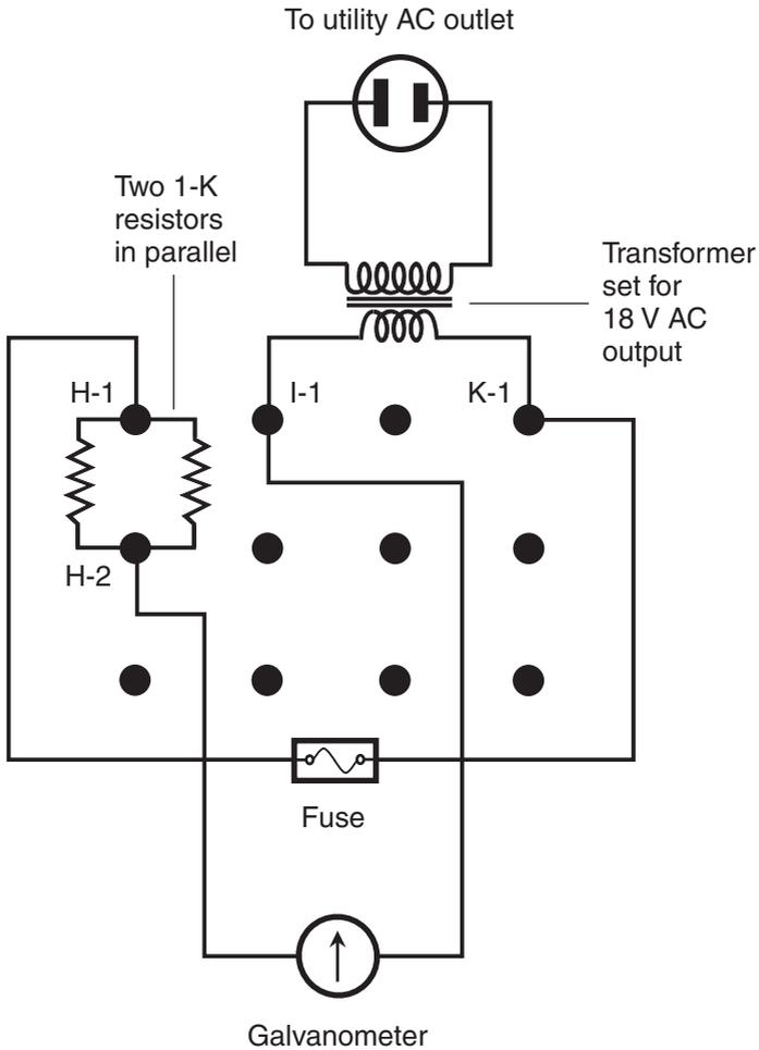
**Figure AC5-2** Suggested breadboard arrangement for testing a galvanometer with AC. The resistors should be rated at  $\frac{1}{2}$  W, and the transformer should be set for 18 V output. Black dots represent breadboard terminals. Note that when two lines (representing wires) intersect in a circuit diagram without a dot, the wires are not meant to be connected to each other at the point of crossing.
