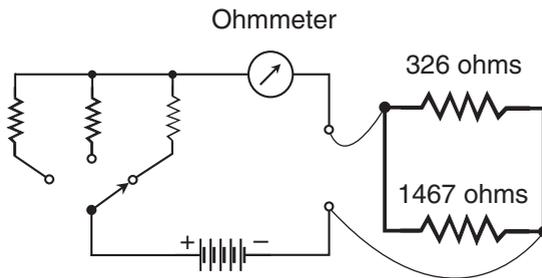
Figure DC10-2 Parallel combination of 326-ohm and 1467-ohm resistances.
