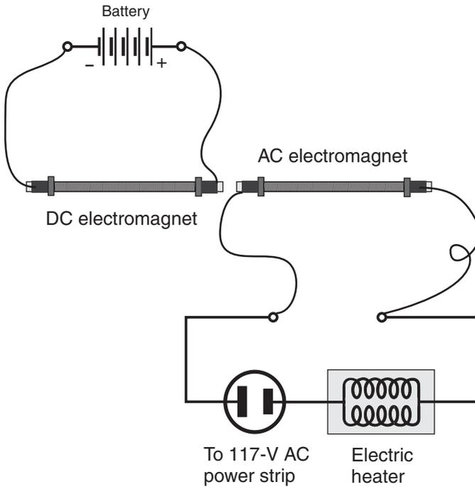
**Figure MAG14-2** *Reversing the DC electromagnet's polarity has no effect on its behavior near the AC electromagnet.*
