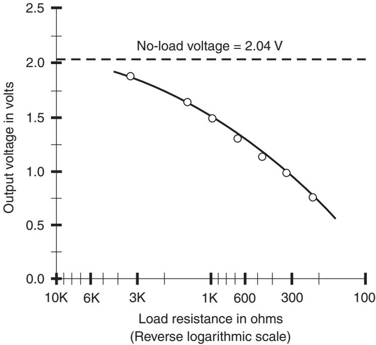
**Figure DC14-5** Output voltage versus load resistance for the resistive voltage divider. These are my results. The dashed line shows the open-circuit (no-load) voltage. Open circles show measured voltages under various loads. The solid curve approximates the circuit's characteristic function.
