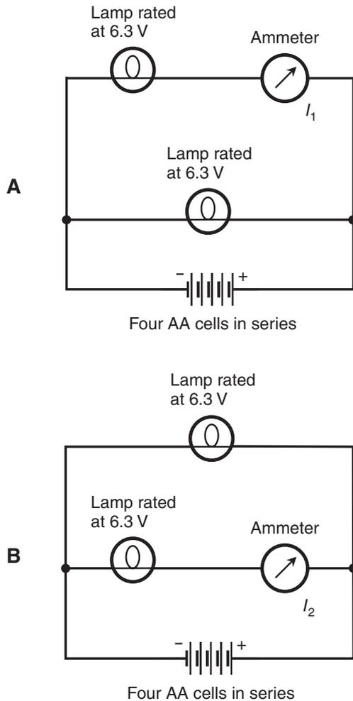
**Figure DC20-1** At A, measurement of current  $I_1$  through the "farther-from-battery" of two "identical" lamps in parallel (called F, rated at 6.3 V). At B, measurement of current  $I_2$  through the "closer-to-battery" lamp (called C, also rated at 6.3 V).
