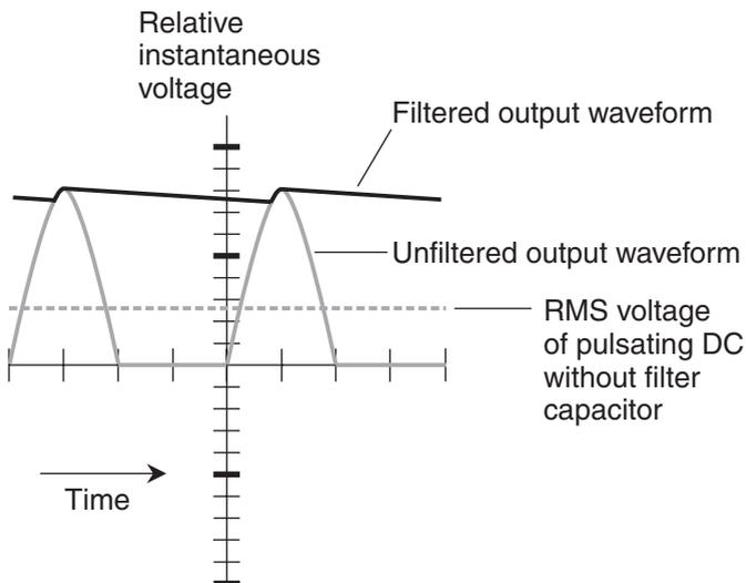
**Figure AC8-2** A filter capacitor charges up to the peak rectifier output voltage with each DC pulse. If the load resistance is high or infinite, the capacitor holds most or all of its charge, so the filtered output voltage is much higher than the RMS output voltage in the absence of the capacitor.
