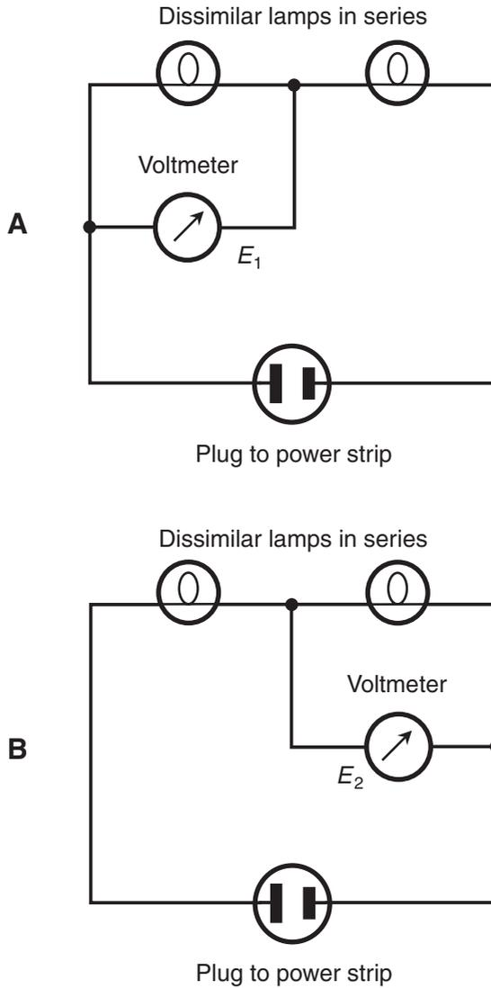
**Figure AC3-1** At A, measurement of voltage  $E_1$  across the bulb in the left-hand of two dissimilar lamps in series (called  $L$ ). At B, measurement of voltage  $E_2$  across the bulb in the right-hand lamp (called  $R$ ).
