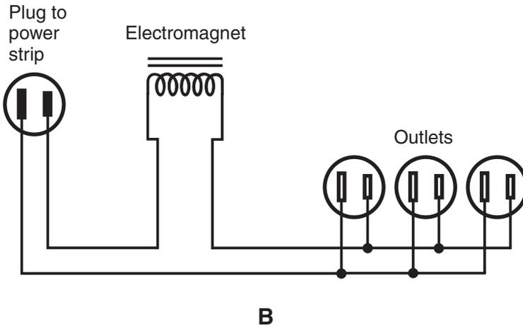
**Figure MAG12-1** Extension-cord modification to connect electromagnet in series with AC outlet. Twist and insulate the splices (drawing A) before you connect the assembly to the power source. Illustration B shows a schematic of the complete system.
