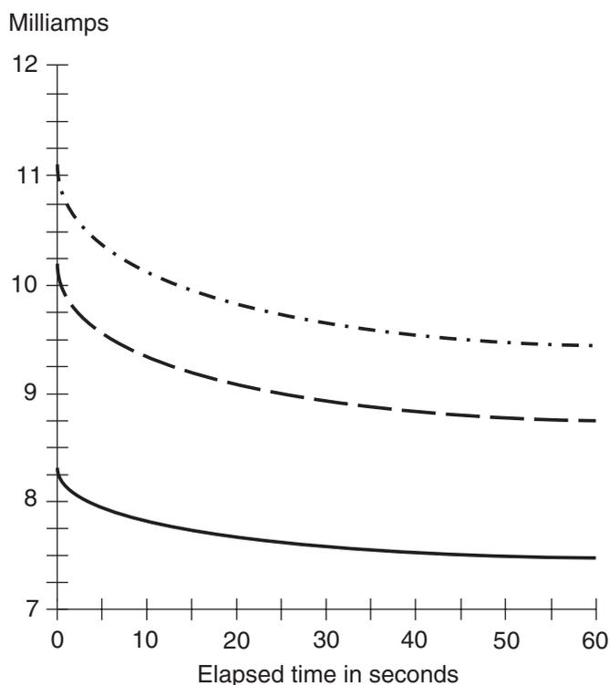
**Figure DC4-3** *Graphs of maximum deliverable currents as functions of time for various amounts of salt dissolved in 12 fluid oz (0.36 L) of vinegar. Lower (solid) curve: one rounded teaspoon of salt. Middle (dashed) curve: two rounded teaspoons of salt. Upper (dashed-and-dotted) curve: three rounded teaspoons of salt.*
