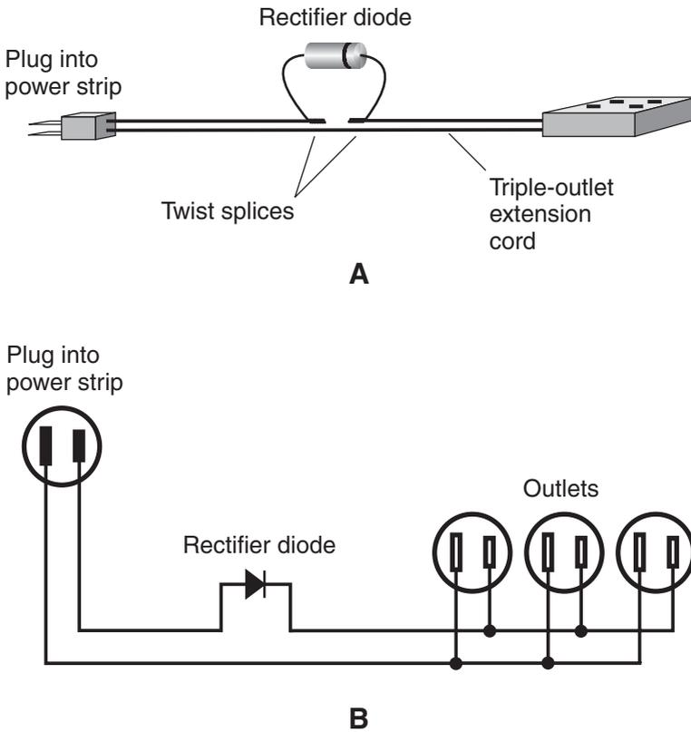
**Figure AC4-1** Drawing A is a pictorial diagram showing the construction of the rectifier cord. The twist splices must be completed, and insulated with electrical tape, before the assembly is connected to any source of power. Drawing B is the schematic circuit diagram.
