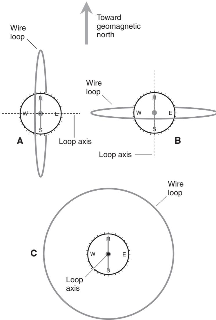
**Figure MAG8-3** *Relative positions of wire loop and compass. At A, loop axis running east-west with compass at center. At B, loop axis running north-south with compass at center. At C, loop axis oriented vertically with compass at center. (All views are looking straight down at the compass.)*
