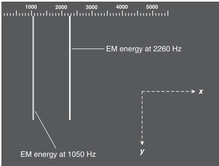
**Figure AC18-2** *The DigiPan display system. The horizontal or  $x$  axis portrays frequency. The vertical or  $y$  axis portrays time. The EM-field “signals” show up as steadily lengthening vertical lines. This drawing shows two hypothetical examples.*
