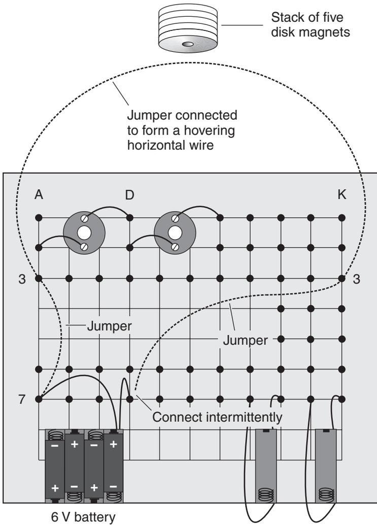
**Figure MAG6-1** Arrangement for observing the effect of magnetic force on a current-carrying wire.
