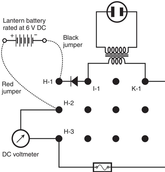
**Figure AC9-2** Measurement of the open-circuit pulsating DC output voltage from the transformer-diode-battery combination with the battery connected “forward” so its voltage adds to the rectified voltage.
