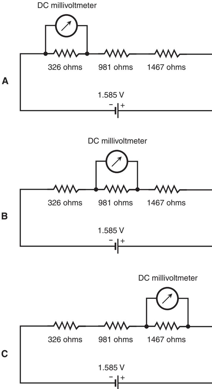
**Figure DC8-2** Schematic diagrams of the arrangements I used to measure the voltage produced by a current of  $553 \mu\text{A}$  through a 326-ohm resistance (A), a 981-ohm resistance (B), and a 1467-ohm resistance (C).
