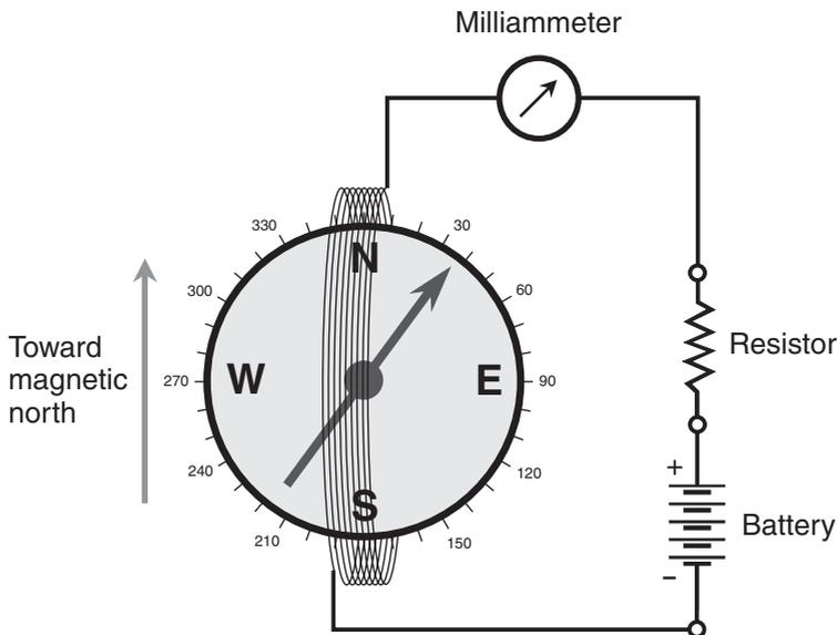
**Figure DC22-3** Arrangement for testing the galvanometer. Be sure that the compass needle points exactly toward N on the scale under no-current conditions, and deflects toward the east of N when current flows through the coil.
