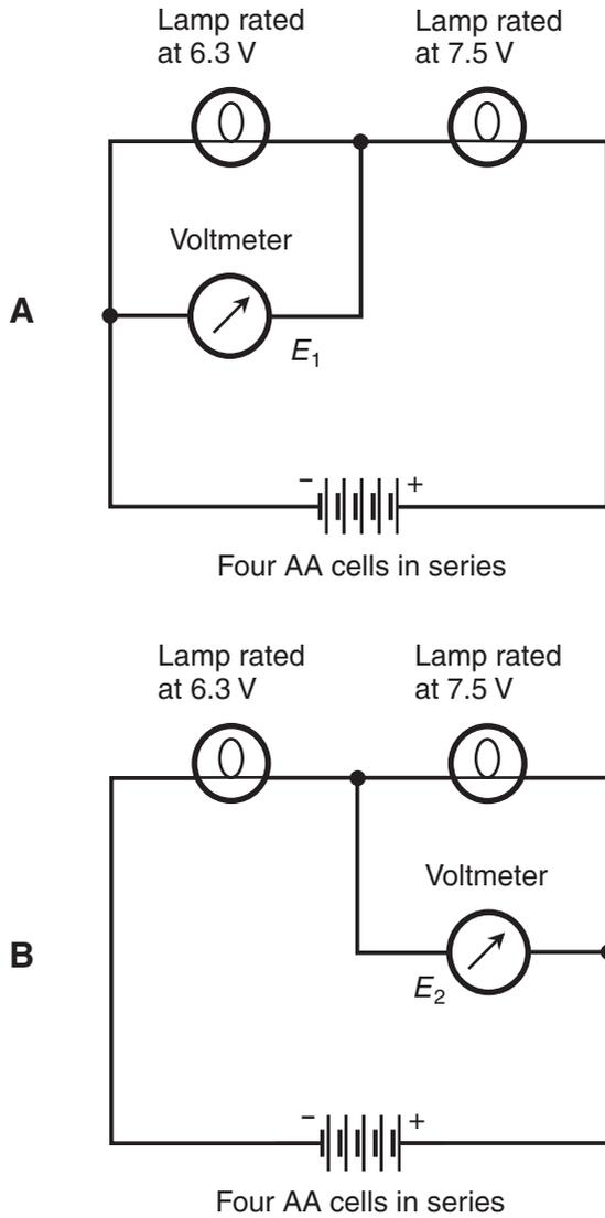
**Figure DC19-1** At A, measurement of voltage  $E_1$  across the more negative of two dissimilar lamps in series (called N, rated at 6.3 V). At B, measurement of voltage  $E_2$  across the more positive lamp (called P, rated at 7.5 V).
