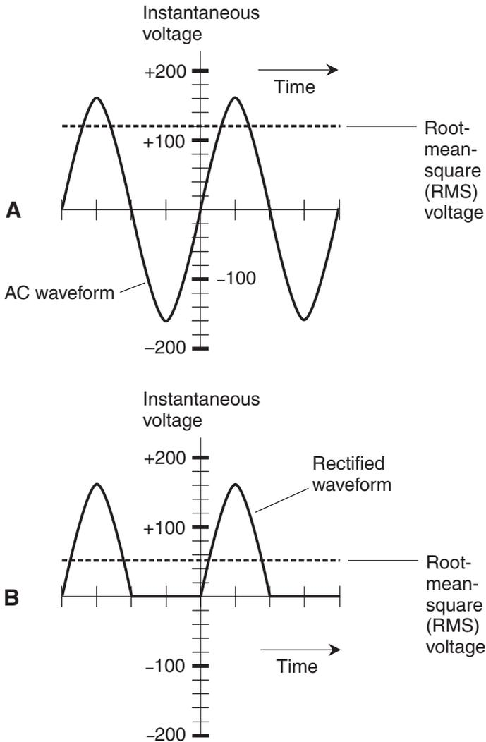
**Figure AC4-2** *Half-wave rectification. At A, the AC waveform as it appears at the power strip. At B, the output waveform as it appears at the cord outlets and across the lamp. Dashed lines indicate root-mean-square (RMS) or effective voltages.*
