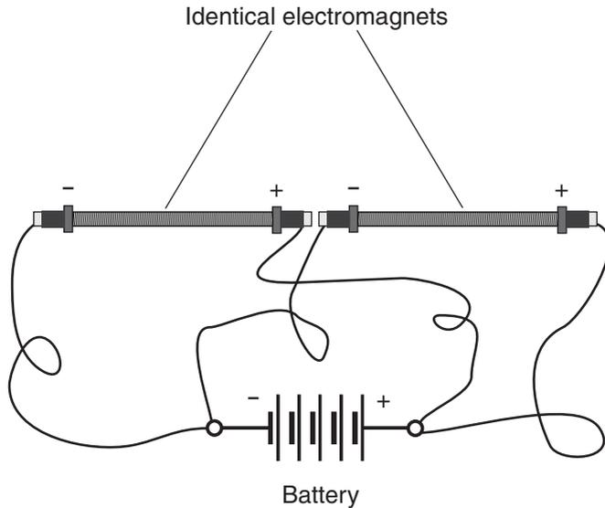
**Figure MAG11-1** *Electromagnets placed end-to-end with opposite poles in proximity.*
