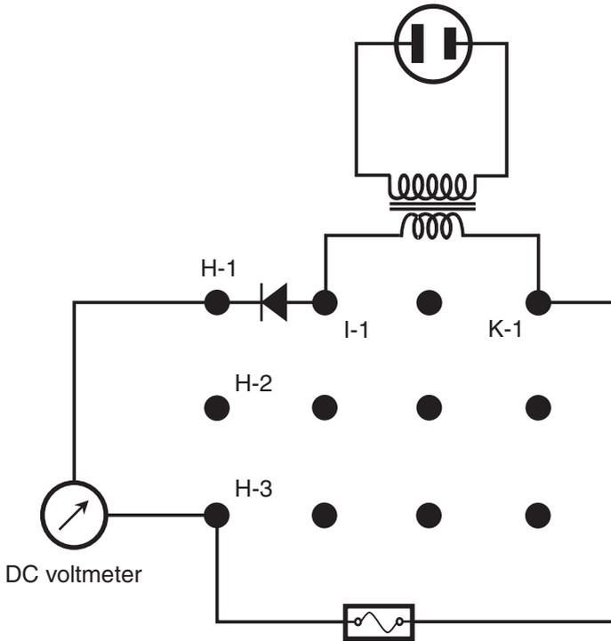
**Figure AC9-1** *Measurement of the open-circuit pulsating DC output voltage from the transformer-diode combination alone. This is the same circuit that you built according to Fig. AC7-2, but the components are arranged differently to accommodate future tests.*
