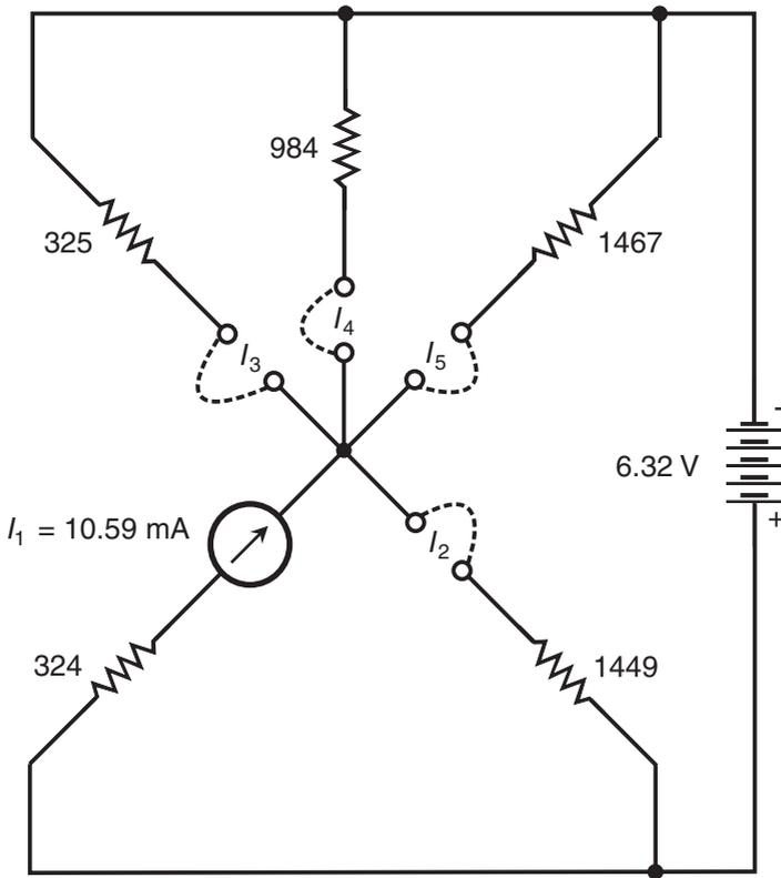
**Figure DC12-3** Network for verifying Kirchhoff's current law. All resistance values are in ohms. The battery voltage, the current  $I_1$ , and the resistances are the values I measured. Dashed lines show interconnections with jumpers.
