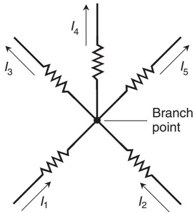
**Figure DC12-2** According to Kirchoff's current law, the sum of the currents flowing into any branch point is equal to the sum of the currents flowing out of that branch point. In this example,  $I_1 + I_2 = I_3 + I_4 + I_5$ .
