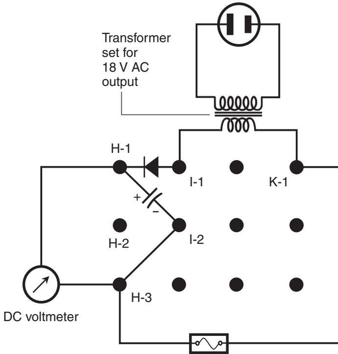
**Figure AC10-1** *Measurement of the open-circuit filtered DC output voltage from the transformer-diode-capacitor combination alone. This is the same circuit that you built according to Fig. AC8-1, but the components are arranged differently to accommodate future tests.*
