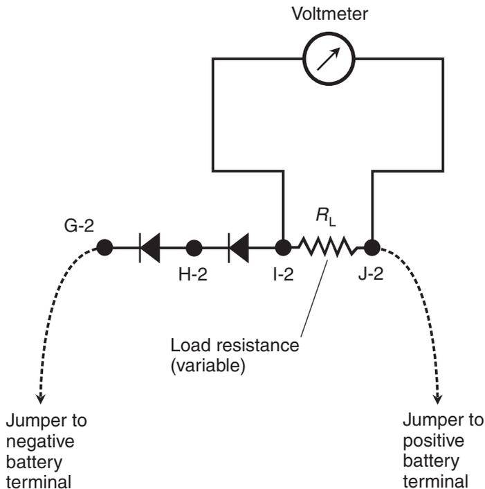
**Figure DC15-3** Suggested arrangement for measurements of the voltages across the load resistance in a two-diode voltage reducer. Solid dots show breadboard terminals. Dashed lines indicate jumpers. Pay attention to the diode polarity! The cathodes should go toward the negative battery terminal.
