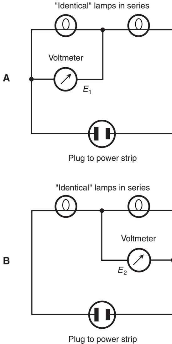
**Figure AC2-2** At A, measurement of voltage  $E_1$  across the bulb in the left-hand of two “identical” lamps in series (called L). At B, measurement of voltage  $E_2$  across the bulb in the right-hand lamp (called R).
