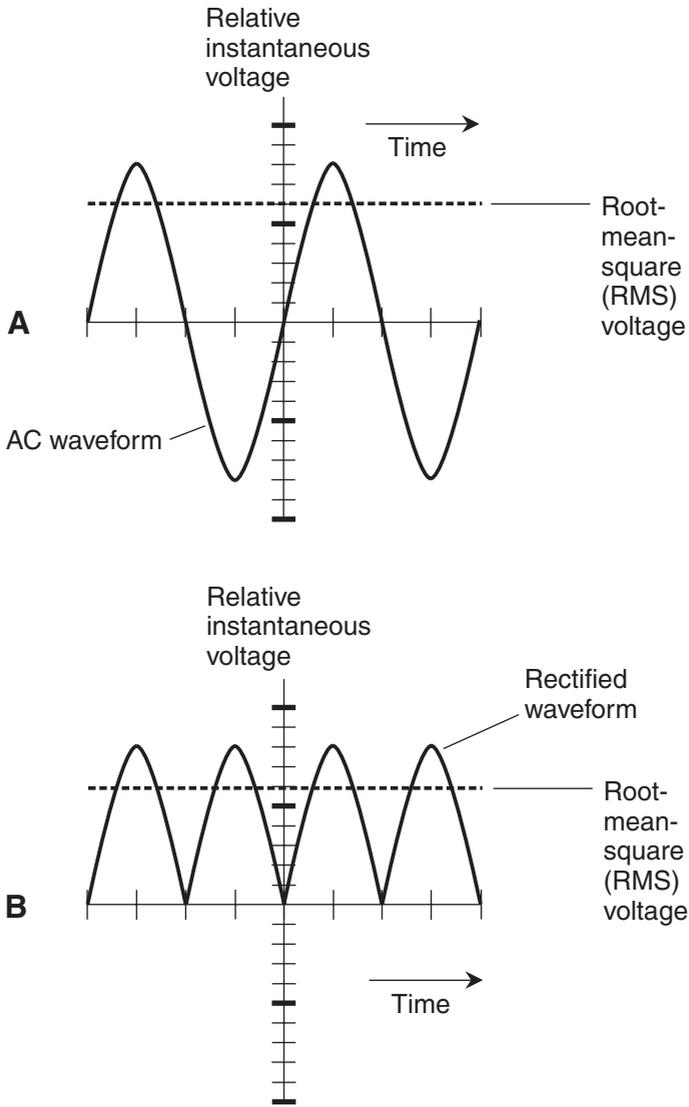
**Figure AC13-1** Full-wave rectification. At A, the AC waveform as it appears at the power strip. At B, the pulsating DC waveform as it appears at the output of the rectifier. Dashed lines indicate root-mean-square (RMS) or effective voltages.
