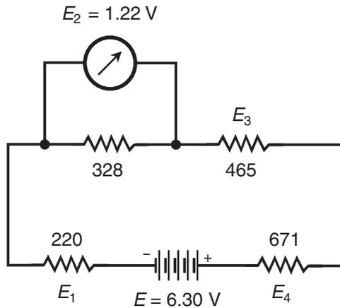
**Figure DC13-3** Network for verifying Kirchhoff's voltage law. All resistance values are in ohms. The battery voltage  $E$ , the voltage across the second resistor, and the resistances are the values I measured.
