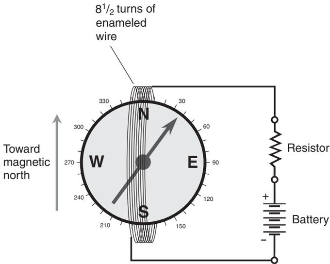
**Figure DC22-1** *The galvanometer and associated circuitry. The compass must lie flat on a horizontal surface, and must be placed so the needle points toward N (magnetic azimuth 0°) when the battery is disconnected.*
