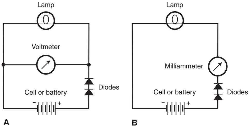
**Figure DC16-2** At A, the arrangement for measuring the voltage across a lamp with diodes in series. At B, the arrangement for measuring the current through a lamp with diodes in series. Pay attention to the diode polarity!
