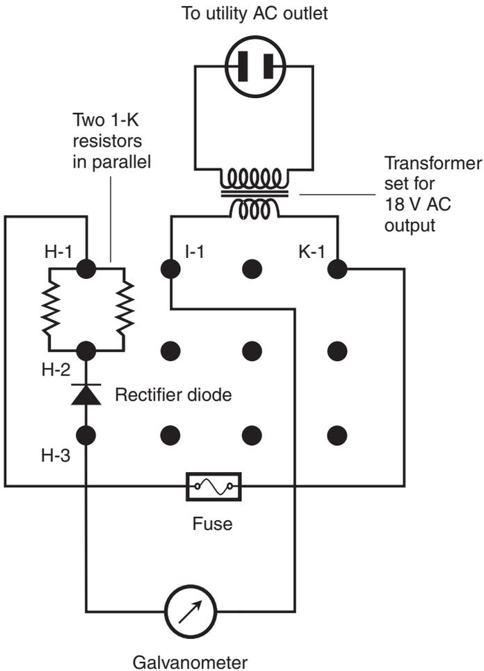
**Figure AC6-1** Suggested breadboard arrangement for testing a galvanometer with diode-rectified AC. The resistors should be rated at  $\frac{1}{2}$  W, and the transformer should be set for 18 V output. Black dots represent breadboard terminals.
