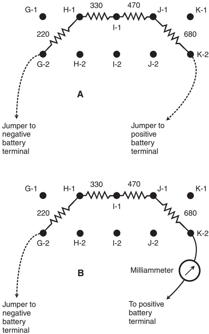
**Figure DC14-2** At A, suggested arrangement for measurements of the voltages across individual resistors. All resistance values are in ohms. Solid dots indicate terminals. Dashed lines indicate jumpers. At B, suggested arrangement for measurement of current through the network.
