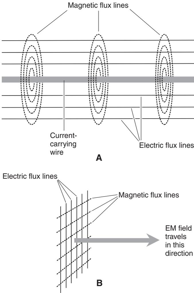
**Figure AC18-1** At A, the electric and magnetic lines of flux around a straight, current-carrying wire. At B, the flux lines far from a current-carrying wire. The EM field travels straight away from the wire, in a direction perpendicular to both sets of flux lines.
