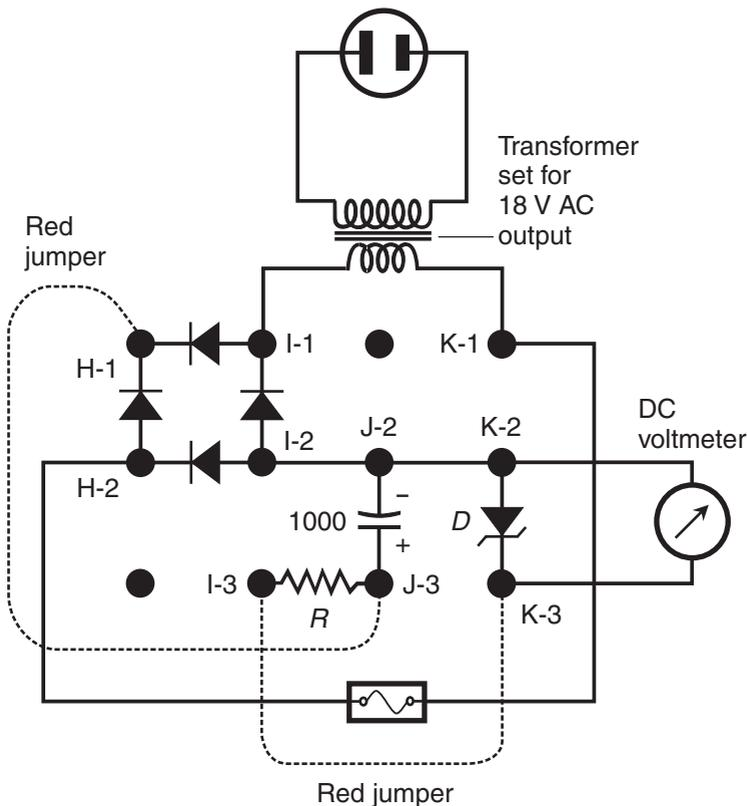
**Figure AC16-1** Addition of a current-limiting resistance  $R$  and a Zener diode  $D$  to regulate the DC output voltage from a filtered full-wave rectifier. The meter is connected to measure the regulated output voltage under no-load conditions.
