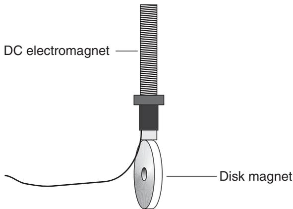
**Figure MAG10-2** *Disk magnet “hanging” from the end of an electromagnet’s core when no current flows through the coil. What will happen when you connect the electromagnet’s coil to a lantern battery?*
