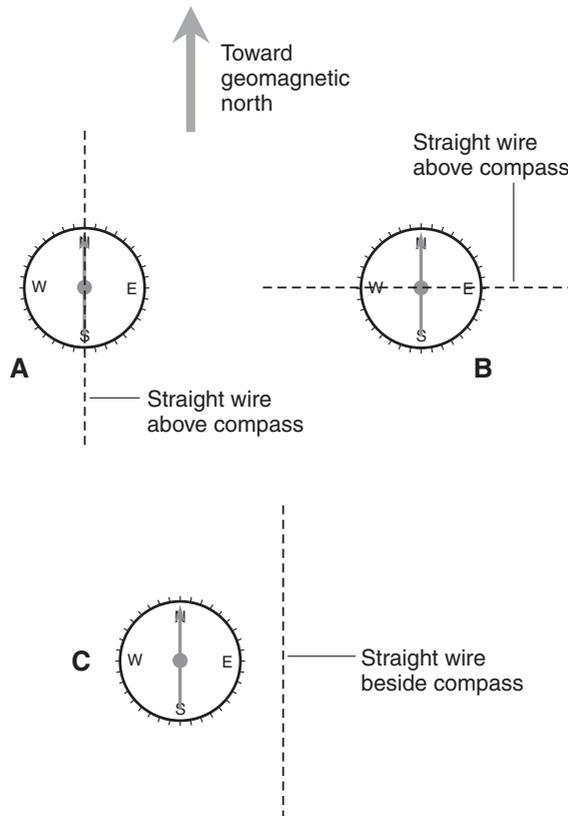
**Figure MAG7-4** *Relative positions of straight wire and compass. At A, wire running north-south above compass. At B, wire running east-west above compass. At C, wire running north-south beside compass.*
