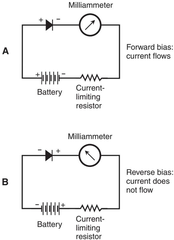
**Figure DC15-2** Series connection of a battery, a resistor, a current meter, and a diode. At A, forward bias causes current to flow if the voltage is at least equal to the forward breakover. At B, reverse bias results in no current through the diode, unless the voltage is very high.
