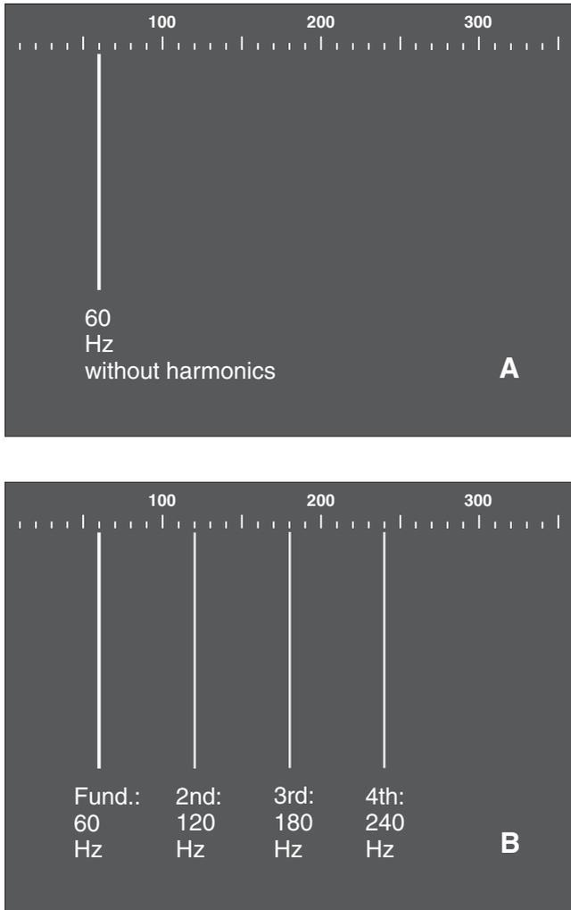
**Figure AC18-3** At A, a spectral diagram of pure, 60-Hz EM energy. At B, a spectral diagram of 60-Hz energy with significant components at the second, third, and fourth harmonic frequencies.
