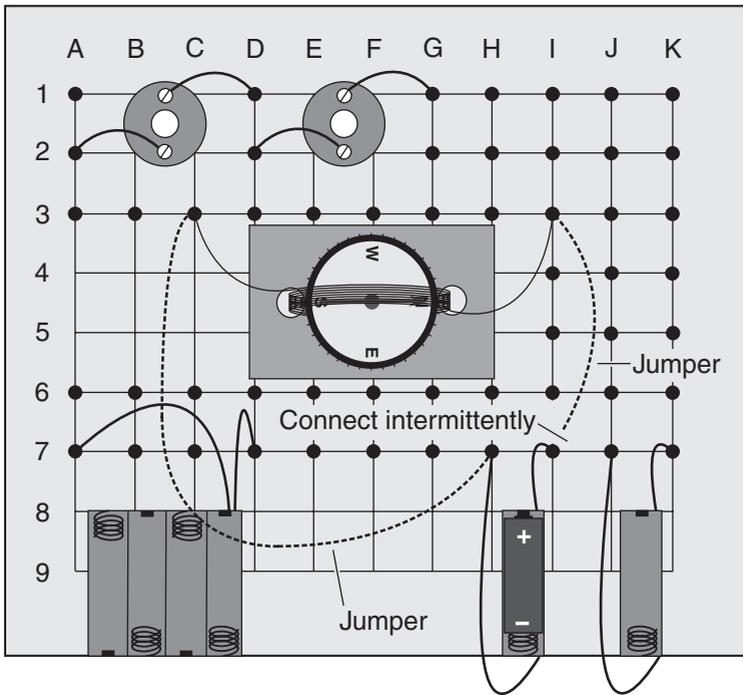
**Figure DC22-2** Suggested placement of the galvanometer on the breadboard. The jumper for the positive cell terminal is normally disconnected. This jumper should never be connected to the cell for more than a couple of seconds at a time.
