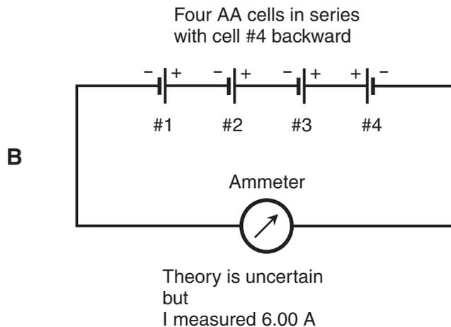
**Figure DC3-2** When I connected one of the end cells backward, I expected to get 4.6 or 4.7 A, but in real life the current was higher. With the arrangement shown at A, I measured about 6.25 A; with the arrangement shown at B, I measured about 6.00 A.
