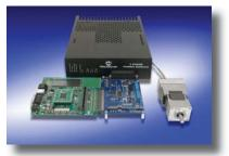
A 3-phase Low Voltage Power Module with Explorer 16 Board, Motor Control Interface Board and a Hurst Motor are shown.
