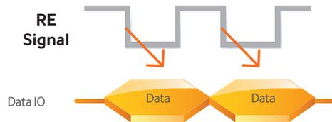
In contrast, modern NAND can handle data on “both edges” of its regulatory signal (or strobe, as it is known). This concept is similar to how DDR RAM works (DDR stands for “Double Data Rate”).
