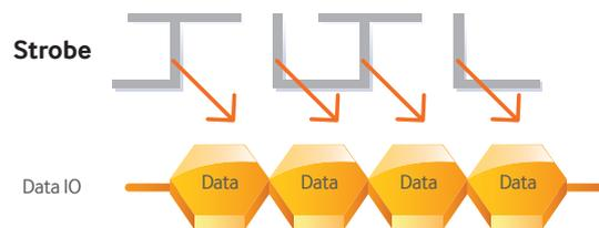
Toggle DDR NAND works much the same way as the DDR NAND diagram above. The strobe that is used to coordinate the NAND operations has rhythmic rises and falls, and Toggle DDR NAND is capable of processing data on both the rise and fall.
