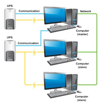
You can even have a UPS that has the serial port connected to a system that it's not feeding. Sometimes a PC will be close to a UPS that needs to be monitored, so it's drafted to supply a serial port for the purpose. This PC may in fact be getting power from some other UPS. This is not a problem.
