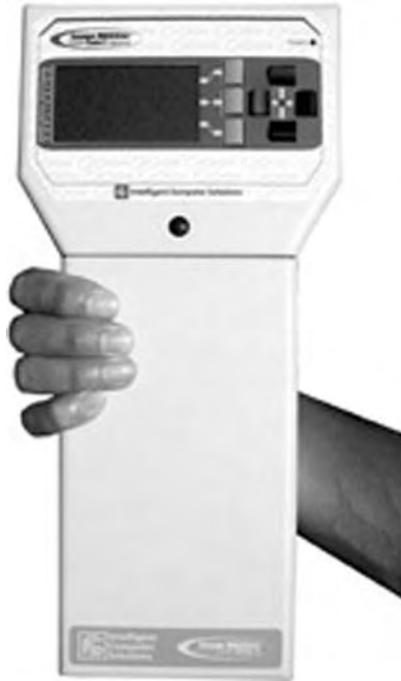
**Figure 3.4** ICS Image MASSter Solo 2 hand-held forensic unit (Reprinted with permission, 2002.)
