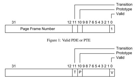
Figure 2: PDE and PTE bits relevant to address translation
