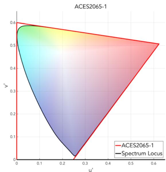
encoding, is capable of capturing all the color nuances of any film stock as easily as it does all the color detail of digital image sensors.
