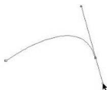
3. Drag the direction line closer to the anchor point to flatten the curve; drag farther away from the anchor point to increase the curve, as shown in Figure 4-5.
