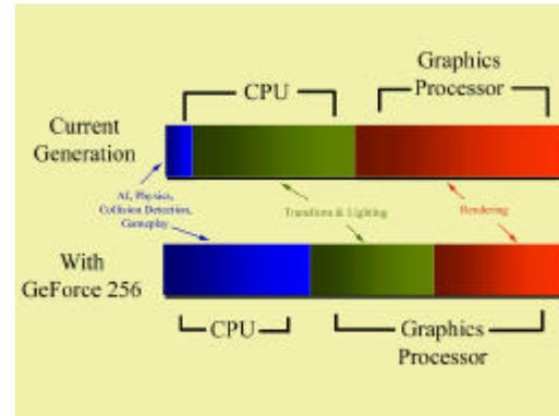
**The GeForce 256 offloads transform and lighting from the host CPU, allowing the CPU to process more game play elements.**
