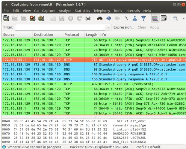
Figure 3: Traffic capture of sqlmap run with DNS exfiltration
