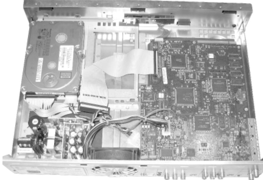
Now to carefully free the cables. If your TiVo had only one drive when it left the factory, the power connector for the second drive should be tied down with cable ties and may be tucked underneath the motherboard. You need to slide it out from under the motherboard and cut those ties; be very careful not to cut any of the wires. Next, if the IDE
