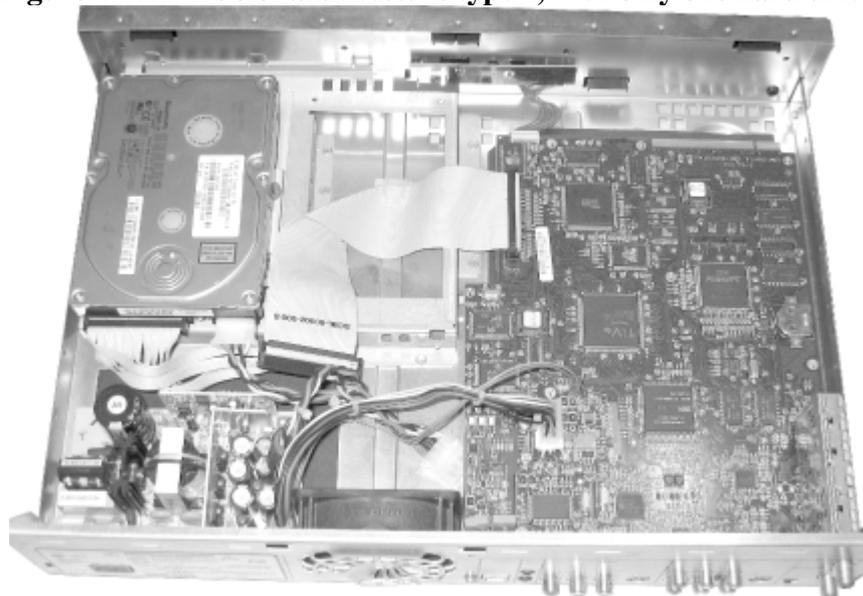
Now to carefully free the cables. If your TiVo had only one drive when it left the factory, the power connector for the second drive should be tied down with cable ties and may be tucked underneath the motherboard. You need to slide it out from under the motherboard and cut those ties; be very careful not to cut any of the wires. Next, if the IDE
