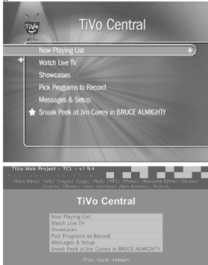
If you click on any link in the Screen emulator, not only will the web page change, but the television screen will also reflect the changes. Those links on the bottom of [Figure 5-22](#) are persistent throughout the entire emulator. You can always hit the button, hit the Back button, or refresh the screen in case the TiVo has changed out from under the web page.
