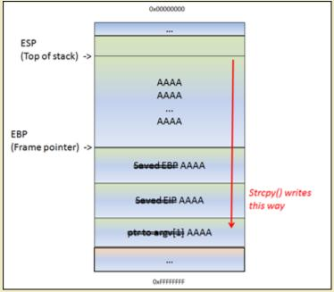
ESP still points at the begin of the string. The strcpy() completes as if nothing is wrong. After the strcpy(), the function ends. And this is where things get interesting. The function epilog kicks in. Basically, it will move ESP back to the location where saved EIP was stored, and it will issue a RET. It will take the pointer (AAAA or 0×41414141 in our case, since it got overwritten), and will jump to that address. So you control EIP
