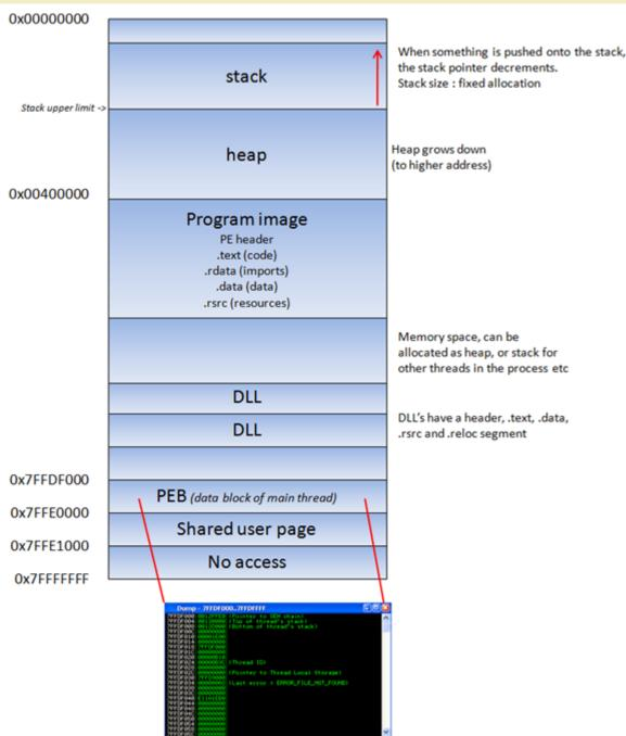
The text segment of a program image / dll is readonly, as it only contains the application code. This prevents people from modifying the application code. This memory segment has a fixed size. The data segment is used to store global and static program variables. The data segment is used for initialized global variables, strings, and other constants.
