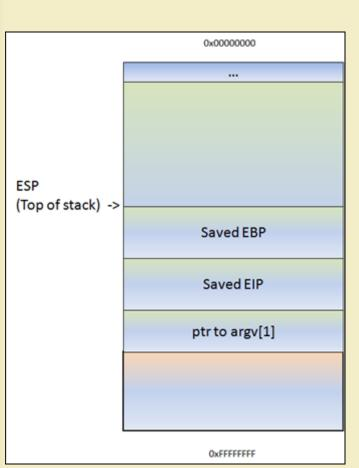
Following the push ebp, the current stack pointer (ESP) is put in EBP. At that point, both ESP and EBP point at the top of the current stack. From that point on, the stack will usually be referenced by ESP (top of the stack at any time) and EBP (the base pointer of the current stack). This way, the application can reference variables by using an offset to EBP.
