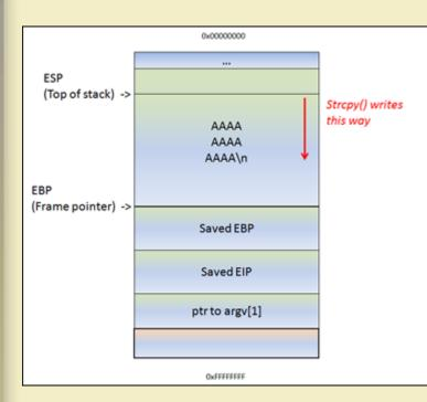
That means... If the data in [Buffer] is somewhat longer than 0×98 bytes, the strcpy() will overwrite saved EBP and eventually saved EIP (and so on). After all, it just continues to read & write until it reaches a null byte in the source location (in case of a string)
