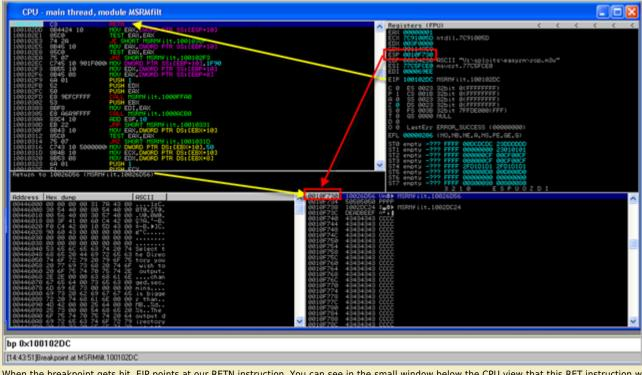
When the breakpoint gets hit, EIP points at our RETN instruction. You can see in the small window below the CPU view that this RET instruction will return to 0x10026D56 (which sits at the top of the stack, the location where ESP point at)
