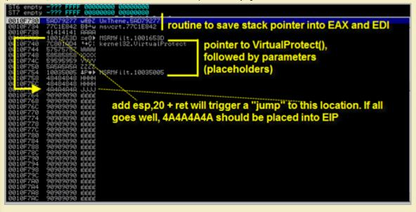
Step through the instructions and watch EAX, EDI and ESP closely. You should see that ESP is pushed onto the stack, placed into EDI. Then EDI is pushed onto the stack and picked up in EAX. Finally  $0 \times 20$  bytes are added to ESP and RET will put 4A4A4A4A in EIP (JJJJ = my \$rop2) Got that? Let's continue.
