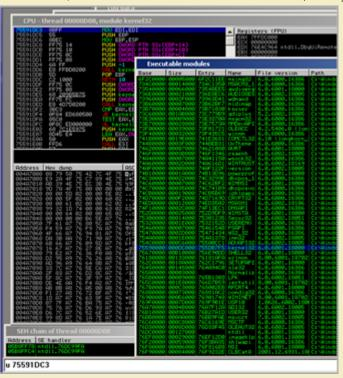
On the stack, the pointer at 0012FF8C is 755DD0E9. If we subtract the offset (0x4B326 bytes) again, we end up at 75591DC3. And that's VirtualProtect! This means that we have found a reliable place to pick up a kernel32 pointer, and found a reliable offset to get to VirtualProtect(). How can we get this value from the stack into a register so we can use it to set up the API call?
