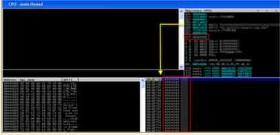
... and ESP points at an address that contains our C's. So far so good, this is a typical direct RET overwrite exploit.
