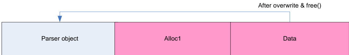
Diagram 17. Chunk overwrite and free
