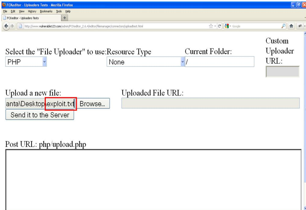
**Step#2:** The attacker clicks on the 'Send it to the Server' button and captures the request in an HTTP proxy:
