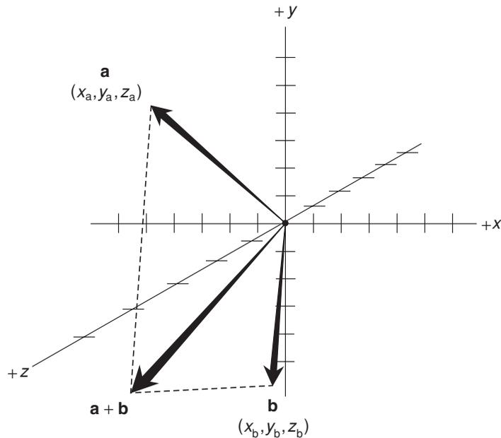
**Fig. 12-3.** Two vectors,  $\mathbf{a}$  and  $\mathbf{b}$ ,  $xyz$ -space. Their sum vector,  $\mathbf{a} + \mathbf{b}$ , is also shown. (The vector-addition parallelogram is distorted by the perspective.)
