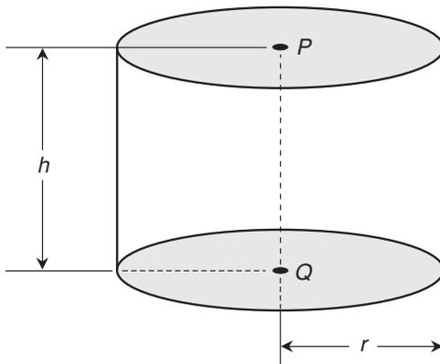
Fig. 9-9. Dimensions of a right circular cylinder.
