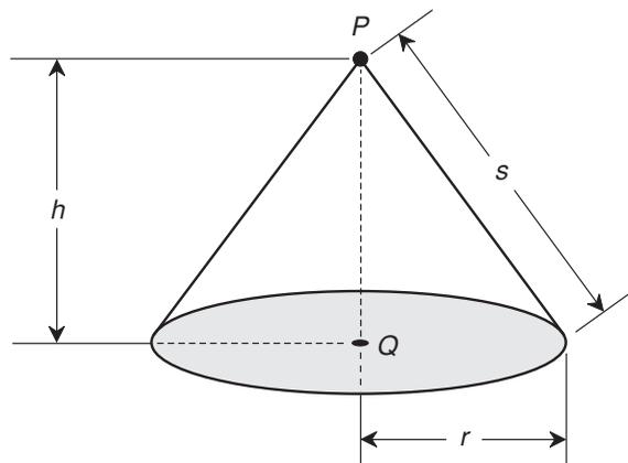
Fig. 9-6. Dimensions of a right circular cone.
