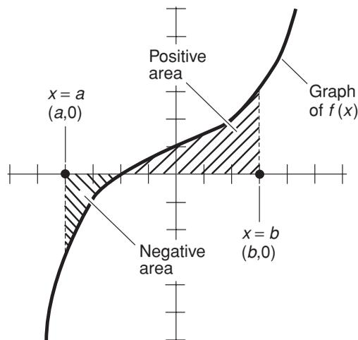
**Fig. 15-1.** A definite integral in the  $xy$ -plane can be represented as the area between the curve and the  $x$  axis, as defined between “vertical lines” passing through two points on the  $x$  axis. In this case the two points are  $(a, 0)$  and  $(b, 0)$ . Areas “above” the  $x$  axis are considered positive. Areas “below” the  $x$  axis are considered negative.
