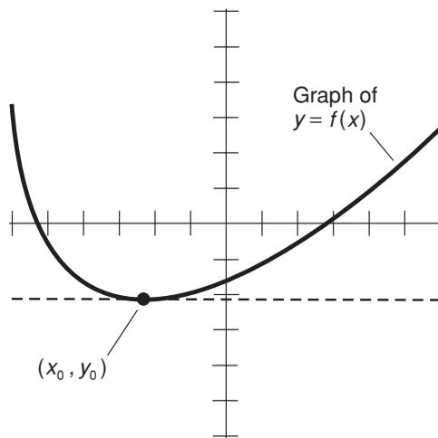
Fig. 14-6. A local minimum value of a function.
