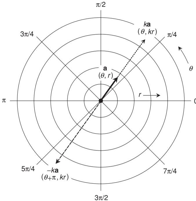
**Fig. 12-8.** Multiplication of a vector  $(\theta, r)$  by a positive real scalar  $k$ , and by a negative real scalar  $-k$ , in the polar plane. Note that the radius of a vector in polar coordinates is not allowed to be negative.
