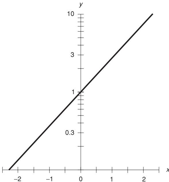
**Fig. 13-8.** Partial semilog graph of the natural exponential function. In this illustration, the  $x$  axis intersects the  $y$  axis at the point where  $y = 0.1$ .
