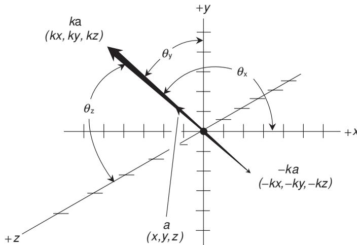
**Fig. 12-9.** Multiplication of a vector by a positive real scalar  $k$ , and by a negative real scalar  $-k$ , in  $xyz$ -space.
