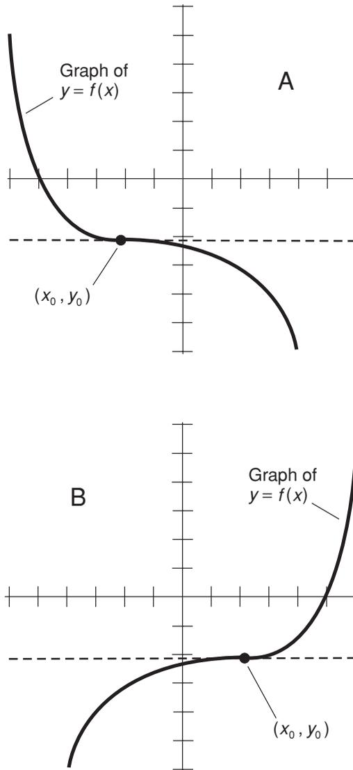
**Fig. 14-7.** Two examples of inflection points. At A, the function generally decreases; at B, the function generally increases. The tangent lines at the inflection points shown here both happen to have slope 0, but this is a mere coincidence.
