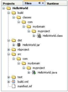
Figure 2-8 Files window "physical" view of the HelloWorld project
