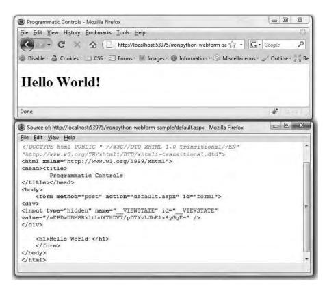
Figure 9-4. The HtmlGenericControl renders as the type we specified as a parameter.
