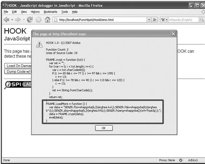
Figure 7-8 HOOK enumerates the window object and extracts the two user-defined functions in the FRAME framework.
