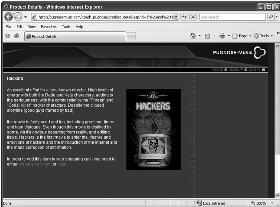
**Figure 3-10** The server's response to the always-true injected XPath query
