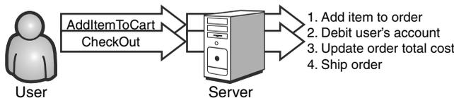
Figure 5-5 An attacker exploits a race condition by calling `AddItemToCart` and `Checkout` almost simultaneously.
