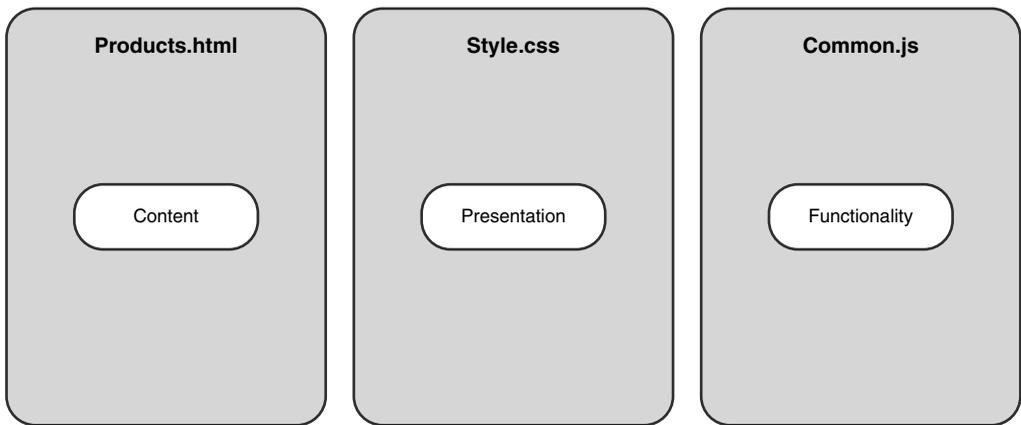
**Figure 12-3** Storing content, presentation, and functionality in separate files eases maintenance and user experience issues.
