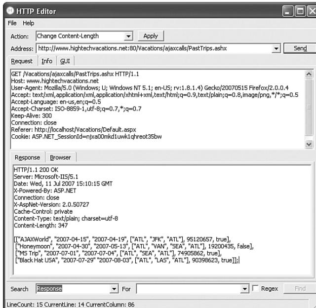
**Figure 7-11** The Ajax endpoint `PastTrips.aspx` returns a nested JSON array containing a user's past trips booked on *HighTechVacations.net*.
