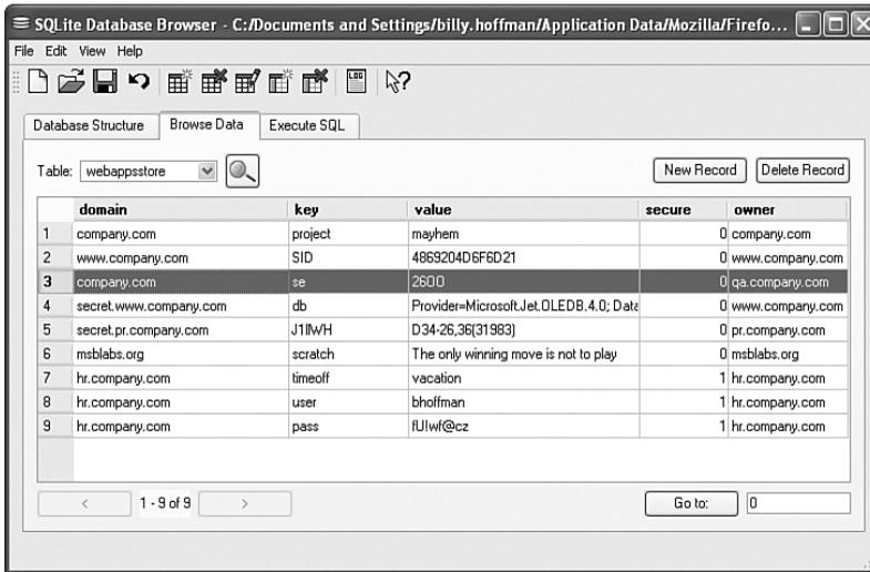
Figure 8-20 Mozilla implements global storage as an easily editable SQLite database.
