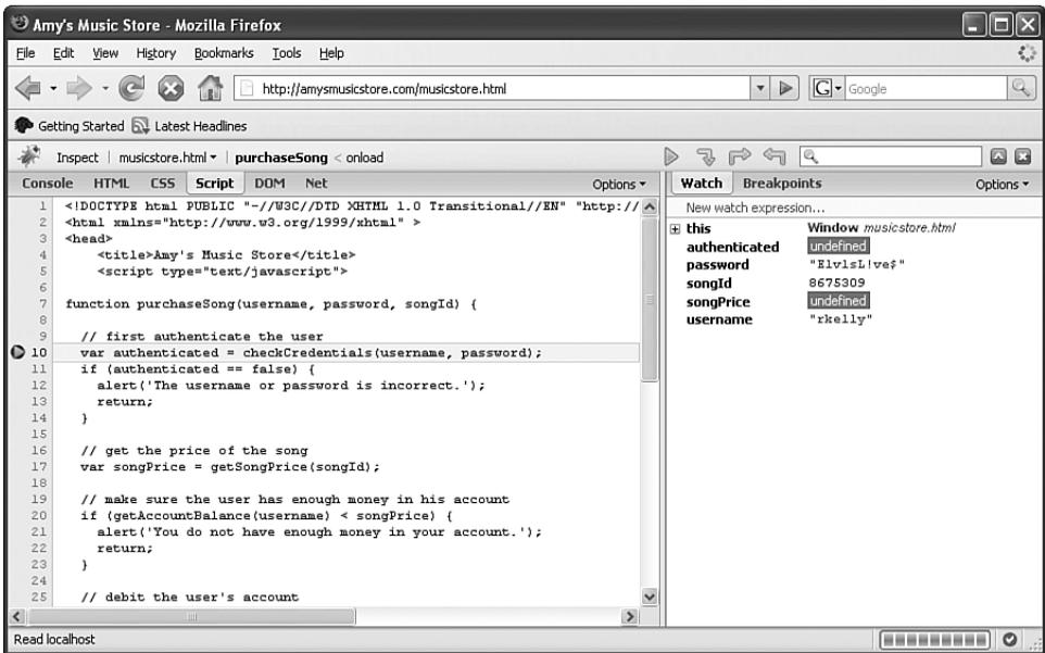
Figure 6-9 Attaching a breakpoint to JavaScript with Firebug
