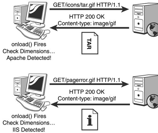
**Figure 13-8** JavaScript can test for the existence of well-known images to fingerprint what Web server or Web application is running on a host.
