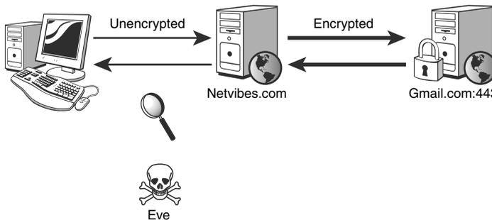
**Figure 11-19** Data transmitted between NetVibes and Gmail is encrypted and cannot be read by an attacker. However, NetVibes retransmits this data to the client unencrypted, degrading security and exposing the data to capture.
