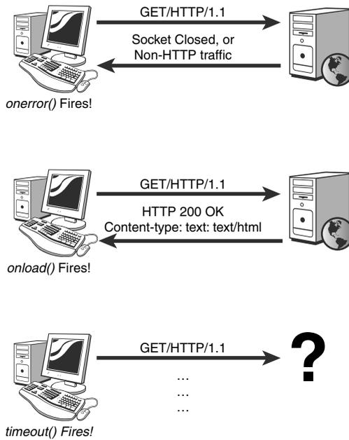
**Figure 13-6** JavaScript can use the Image object to implement a crude version of the ping network utility.
