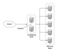
To avoid a central point of failure, the management node itself is clustered, usually in a failover mode with an identical copy of itself (though you can use a DNSRR solution with an IP address for each management node).
