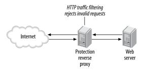
The protection reverse proxy is useful when you must maintain an insecure, proprietary, or legacy system. Direct exposure to the outside world could lead to a compromise, but putting such systems behind a reverse proxy would extend their lifetime and allow secure operation. A protection reverse proxy can also actually be useful for all types of web applications since they can benefit from having an HTTP firewall in place, combined with full traffic logging for auditing purposes.
