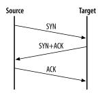
In the normal handshaking process, a host wanting to initiate a connection sends a packet with a SYN flag set. Upon receiving the packet and assuming the server is open for connections on the target port, the target host sends back a packet with flags SYN and ACK set. Finally, the client host sends a third packet with the flag ACK set. The connection is now established until one of the hosts sends a packet with the RST or FIN flag set.
