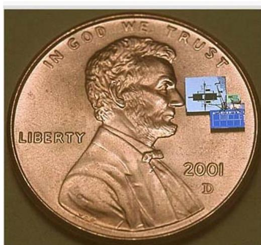
inputs and outputs (dustnetworks.com, 2006). Currently they are highly miniaturized micro-electromechanical devices (MEMs) with imbedded intelligence that pack wireless communication in the digital circuitry (Anonymous 8, 2003; Culler & Mulder, 2004; Warneke & Pister, 2004).
