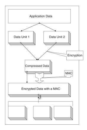
used to verify the integrity of the message included in the transmitted record. The verification is done by the receiving party computing its own value of the MAC and comparing it with that received. If the two values match, this means that data has not been modified during the transmission over the network.
