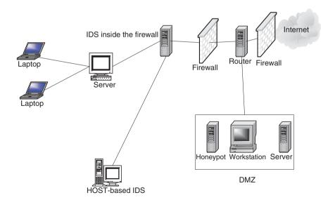
Fig. 13.3 The positioning of a honeypot
