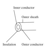
Fig. 1.8 Coaxial Cable
