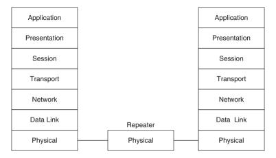
Fig. 1.25 A repeater in an OSI model
