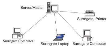
Fig. 1.2 A Centralized network model
