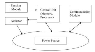
Fig. 19.1 A Wireless Sensor Node
