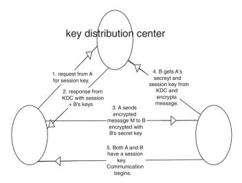
Fig. 11.7 The Working of a KDC
