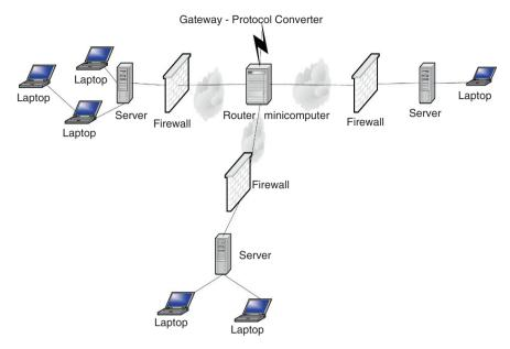
Fig. 1.31 Position of a gateway
