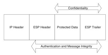
Fig. 17.8 IPSEc's ESP Protocol Protection
