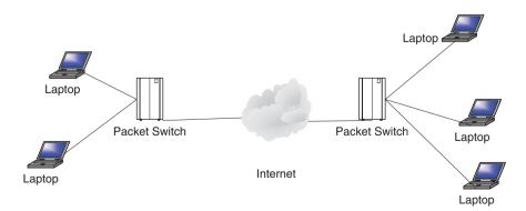
Fig. 1.22 Packet switching networks
