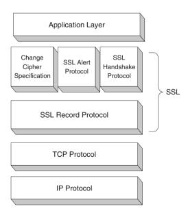
**Fig. 17.4** The SSL Protocol Stack
