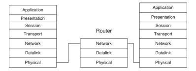
Fig. 1.29 Router in the OSI protocol stack
