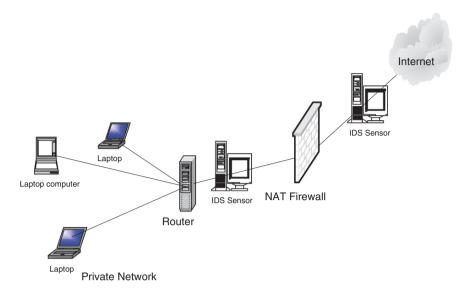
Fig. 12.11 Firewalls with IDS sensors
