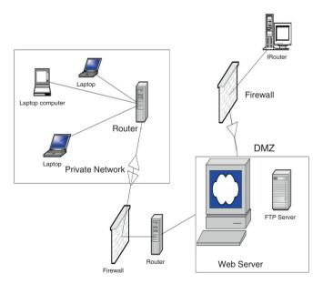
Fig. 12.10 Two firewalls in a network with a DMZ
