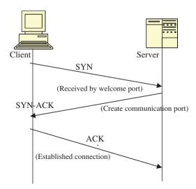
**Fig. 3.1** A three-way handshake
