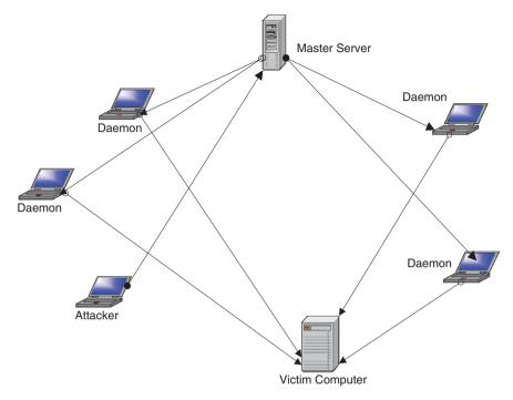
Fig. 3.2 The working of a DDOS attack
