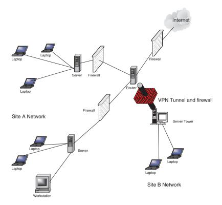
Fig. 12.2 Firewalls in a changing parameter security
