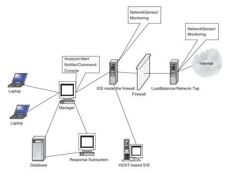
Fig. 13.2 The various places of placing the IDS sensors
