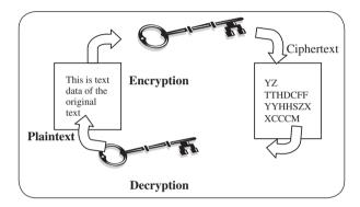
Fig. 11.2 Encryption and Decryption with Symmetric Cryptography
