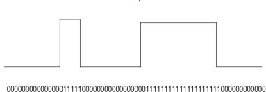
Fig. 1.7 NRZI Nonreturn to zero Invert on ones representation code
