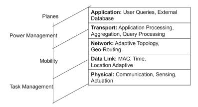
Fig. 19.2 Sensor network protocol stack
