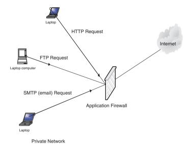
Fig. 12.5 A proxy firewall server
