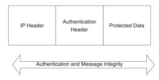
Fig. 17.7 IPSec's AH Protocol Protection
