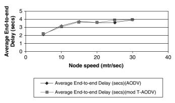
Fig. 4.7. Comparison of average end-to-end delay with node speed
