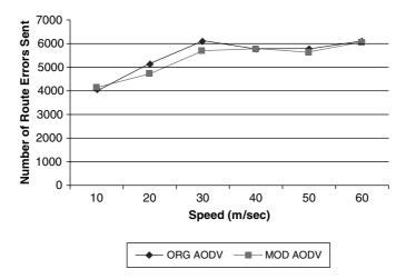
Fig. 4.6. Comparison of route errors with node speed
