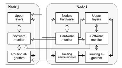
Fig. 10.1. Relationship between software/hardware monitoring and routing
