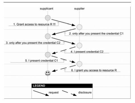
Fig. 2.1. Trust negotiation schema
