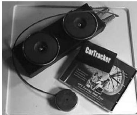
**Figure 14.1** Commercially available covert vehicle tracker using GPS.
