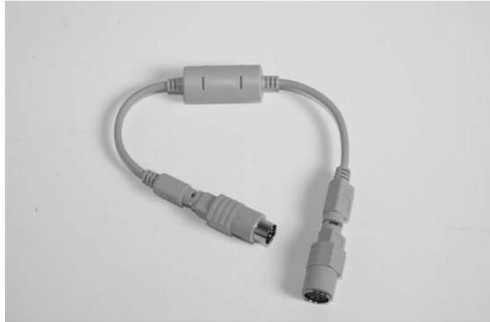
**Figure 4.2** Keyghost keystroke-capturing device with some adaptors.
