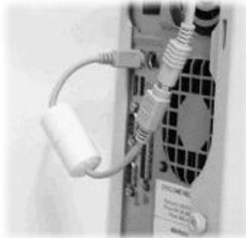
**Figure 4.6** Modified keyboard cable.
