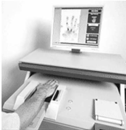
**Figure 15.2** Palm-based biometric reader.
