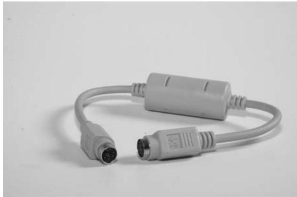
**Figure 4.3** Keyghost keystroke-capturing device without adaptors.
