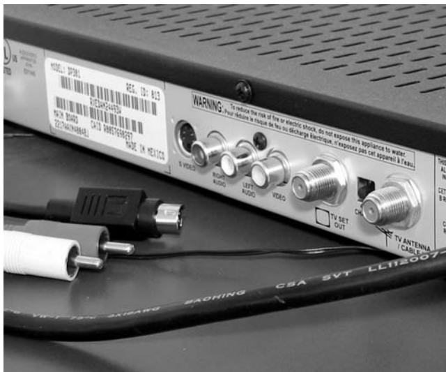
Figure 6-4: Typical set-top box connectors for coaxial TV Out, S-Video Out, and Audio Out.
