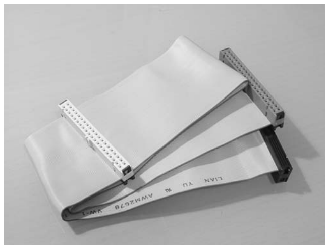
Figure 7-1: IDE cable for adding a second hard drive (note that there are two drive connectors).
