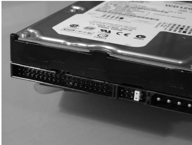
Figure 7-3: Jumper and pins on the back of a hard drive.
