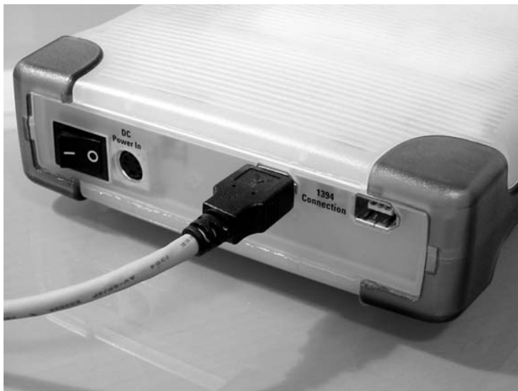
Figure 7-6: The connector on the back of external hard drive.
