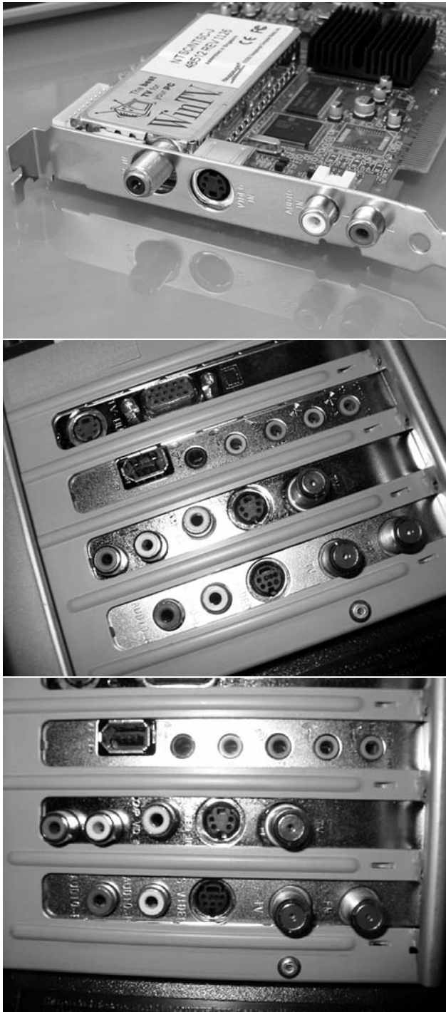
Figure 5-2: FM, coaxial, S-Video, composite video, and audio connectors on a TV tuner card.
