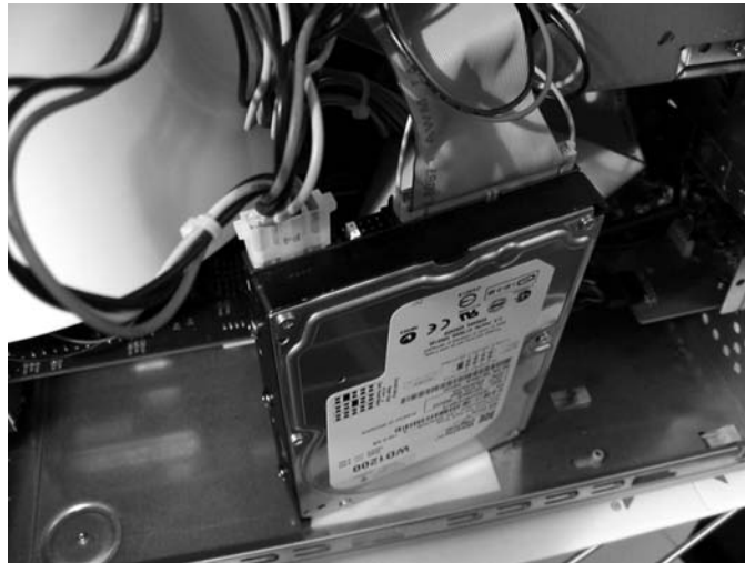
Figure 7-5: IDE cable and power cable connected to the hard drive.
