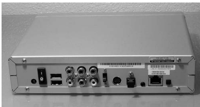
Figure 8-4: Back panel of Extender showing connectors.
