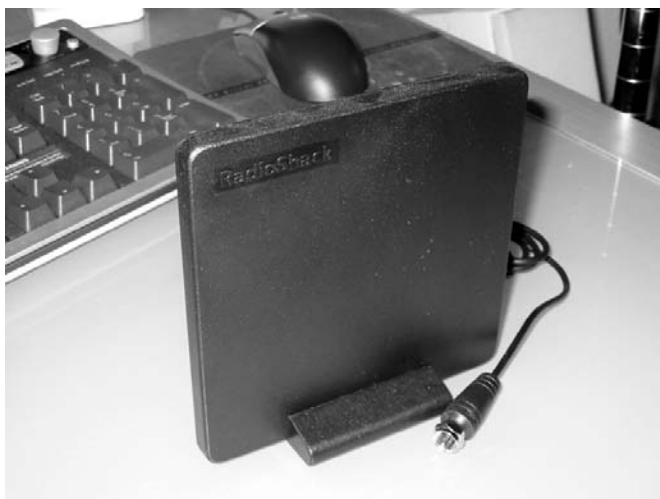
Figure 14-2: A passive FM antenna from Radio Shack with coaxial connector.
