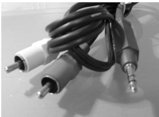
Figure 6-11: \frac{1}{4} " stereo mini plug and RCA-type stereo connectors.
